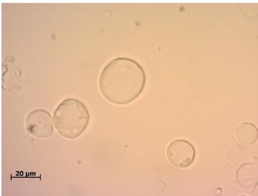
Figure 3-37 Microscope image of a sample mixture of  $1.16 \times 10^6$  (0.025 g) alginate particles and  $1.22 \times 10^{11}$  (25  $\mu\text{L}$ ) chitosan particles for pH 7
