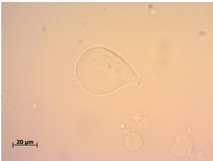
Figure 3-24 Microscope image of a sample mixture of  $2.89 \times 10^5$  (0.00625 g) alginate particles and  $1.22 \times 10^{11}$  (25  $\mu\text{L}$ ) chitosan particles for pH 2.3
