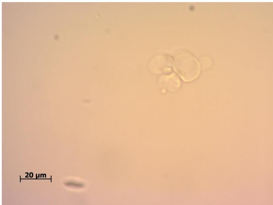
Figure 3-50 Microscope image of a sample mixture of  $5.78 \times 10^5$  (0.0125 g) alginate particles and  $1.22 \times 10^{11}$  (25  $\mu\text{L}$ ) chitosan particles for 0.01 M NaCl
