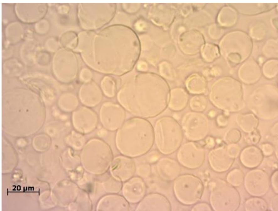
Figure 3-39 Microscope image of a sample mixture of  $4.63 \times 10^6$  (0.1 g) alginate particles and  $1.22 \times 10^{11}$  (25 μL) chitosan particles for pH 7
