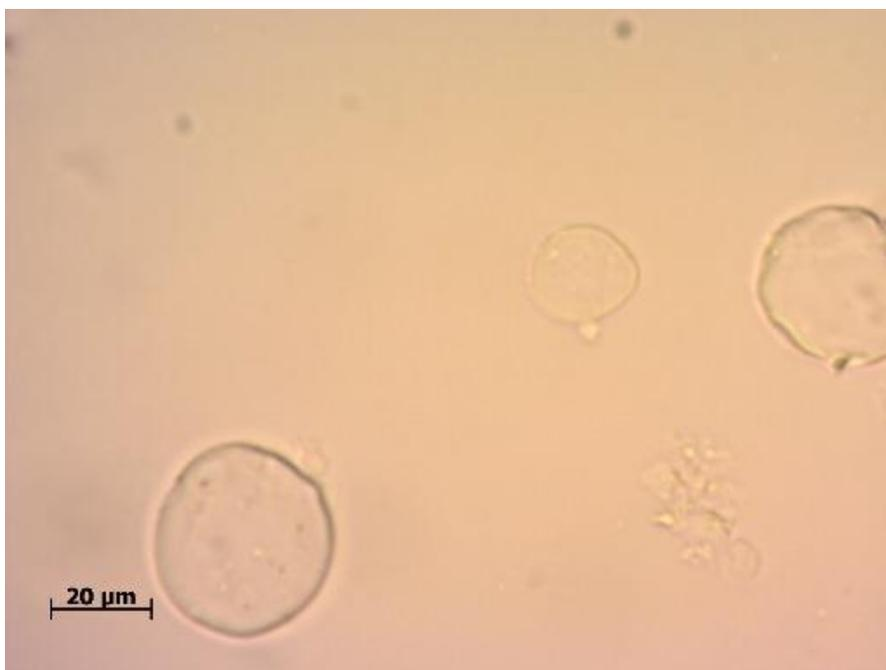
Figure 3-35 Microscope image of a sample mixture of  $2.89 \times 10^5$  (0.00625 g) alginate particles and  $1.22 \times 10^{11}$  (25 μL) chitosan particles for pH 7
