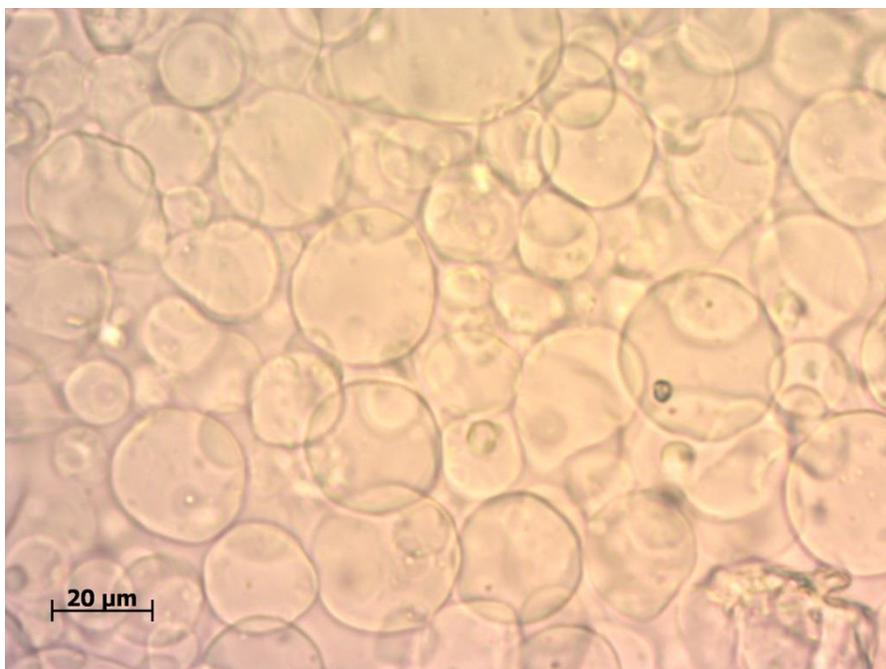
Figure 3-55 Microscope image of a sample mixture of  $1.85 \times 10^7$  (0.4 g) alginate particles and  $1.22 \times 10^{11}$  (25 μL) chitosan particles for 0.01 M NaCl
