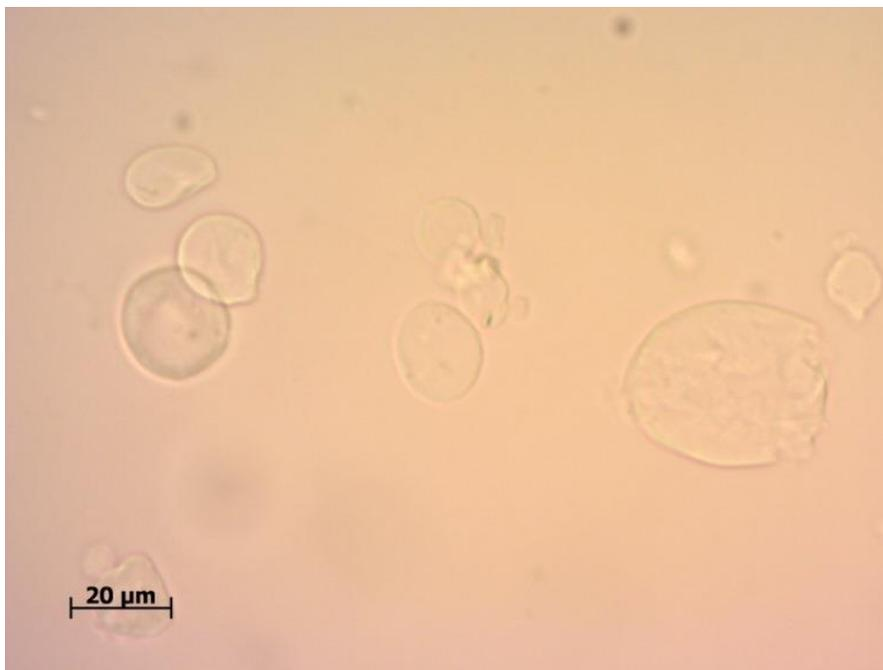
Figure 3-26 Microscope image of a sample mixture of  $1.16 \times 10^6$  (0.025 g) alginate particles and  $1.22 \times 10^{11}$  (25  $\mu\text{L}$ ) chitosan particles for pH 2.3
