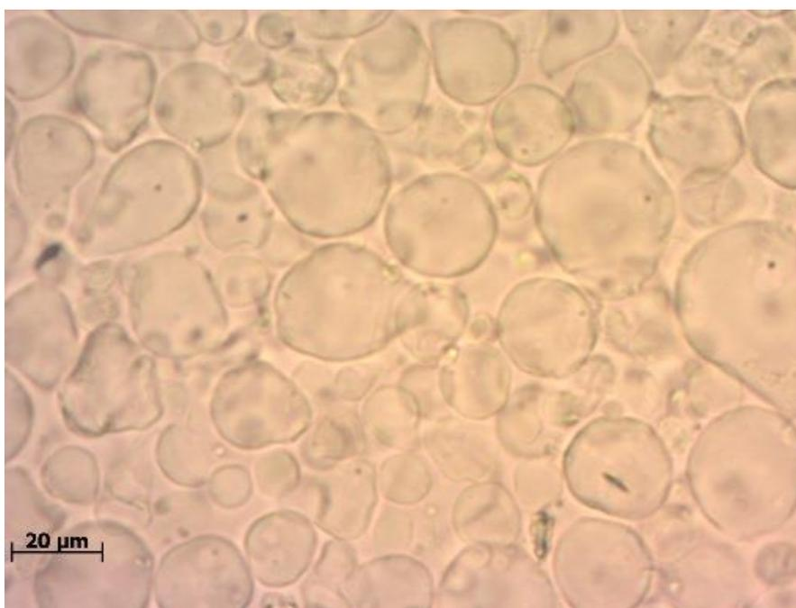
Figure 3-41 Microscope image of a sample mixture of  $1.85 \times 10^7$  (0.4 g) alginate particles and  $1.22 \times 10^{11}$  (25  $\mu\text{L}$ ) chitosan particles for pH 7
