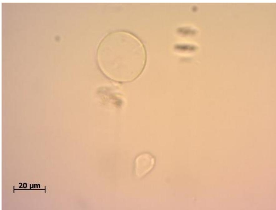
Figure 3-34 Microscope image of a sample mixture of  $1.45 \times 10^5$  (0.003125 g) alginate particles and  $1.22 \times 10^{11}$  (25  $\mu\text{L}$ ) chitosan particles for pH 7
