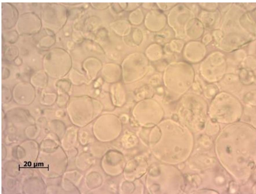
Figure 3-8 Microscope image of a sample mixture of  $1.85 \times 10^7$  (0.4 g) alginate particles and  $1.22 \times 10^{11}$  (25  $\mu$ L) chitosan particles
