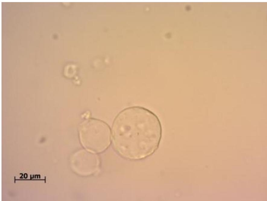
Figure 3-3 Microscope image of a sample mixture of  $5.78 \times 10^5$  (0.0125 g) alginate particles and  $1.22 \times 10^{11}$  (25  $\mu$ L) chitosan particles
