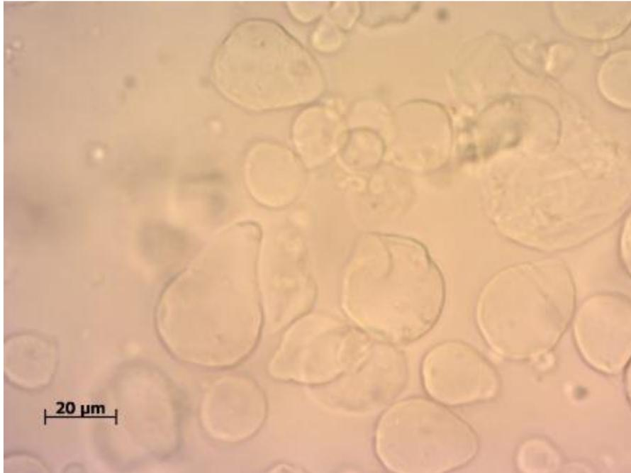
Figure 3-5 Microscope image of a sample mixture of  $2.31 \times 10^6$  (0.05 g) alginate particles and  $1.22 \times 10^{11}$  (25  $\mu$ L) chitosan particles
