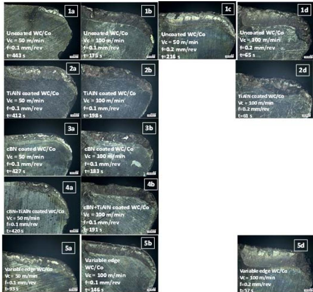
Figure 3.13. Experimental crater wear zones in cutting tools
