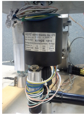
Figure 3.12: Keyo Slip Ring - 25.4mm thru bored, 18 connections
