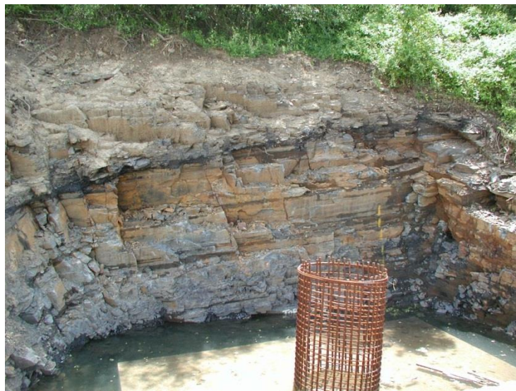
Figure 1.1: Shale mudstone fractured rock where fracture zones are darker units consisting of highly crushed 'coal' units within the sequence. (Photo credit: Pierre Lacombe, USGS)
