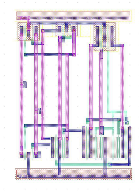
Figure 4.18: Layout of the Pass Transistor PFD
