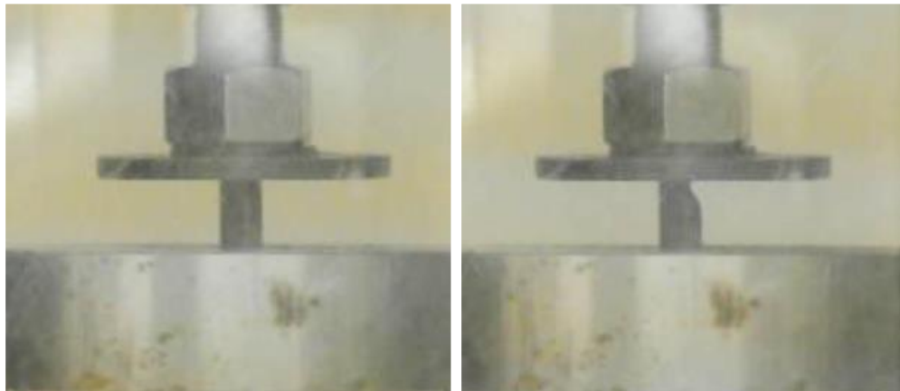
Figure 4-3 – Both image sets are from screenshots of video recorded for each test. The left images are before specimen failures and the right are after specimen failures. Looking at the top image set, at about 21 s into the video for test 3, a shard from the left flies off, and looking at the load and deflection plot for test 3, there is only a minor dip, not a negative deflection at about 0.4 mm. And for the bottom image set, at about 40 seconds into the video for test 5 a large fracture occurs at the upper right corner and flies off. This corresponds with the negative deflection at about 0.5 mm of the load and deflection plot for test 5.
