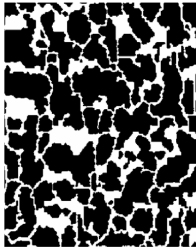
Figure 1-6: Digitized porous microstructure of sandstone computed from X-ray Micro Tomography (XMT). Solid particles are black and pore area is white. Sample dimensions 1418 \mu\text{m} by 1774 \mu\text{m} with a resolution of 24.54 \mu\text{m} . 61
