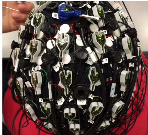
Figure 6.2: ActiCAP on subject showing impedances. Red: high impedance, yellow: medium impedance, green: low impedance
