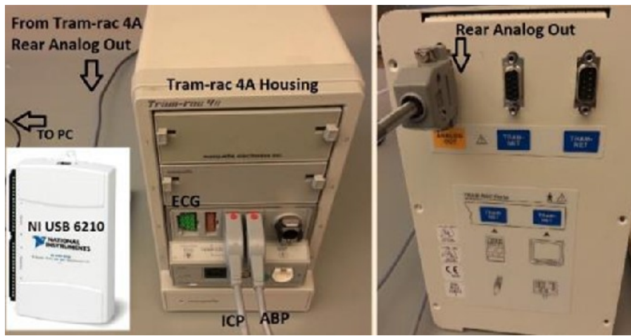
Figure 5: Data collected via analog outputs from the back of a TRAM housing unit: GE Tram-rac 4A; analog outputs were collected using NI-USB 6210 DAQ; signal was sampled at 50 Hz, with a resolution (absolute accuracy) of 1.41 mV at \pm 5 V analog input range, which is equivalent to the pressure resolution of 0.141 mmHg, and capable of detecting \pm 500 mmHg range
