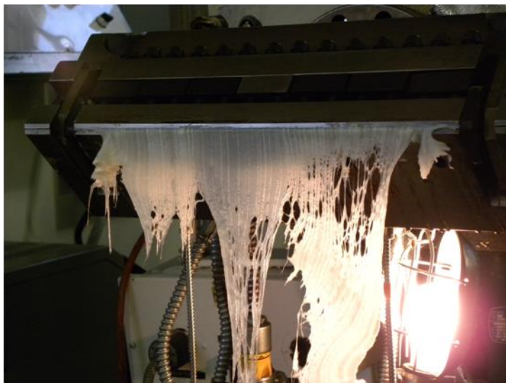
PCL + citric acid upon extrusion
