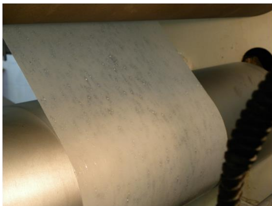
PCL + citric acid upon extrusion
