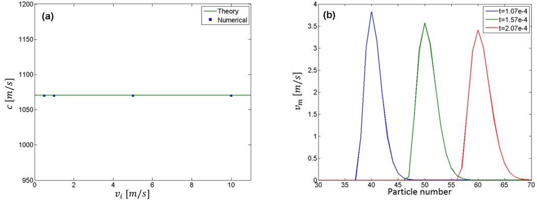
Figure 5: For the harmonic system, plot (a) shows the relationship between the wave propagation velocity  $c$  and the initial velocity of the strikers  $v_i$  in the circumstance  $\hat{J} = 0.14$ . Plot (b) shows the wave front velocity  $v_m$  in the chain at different time in the circumstance  $\hat{J} = 0.07$ ,  $v_i = 5m/s$ .
