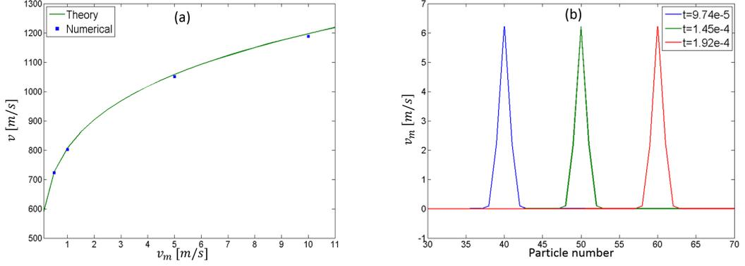
Figure 8: For the hertz system, plot (a) shows the propagation velocity  $v$  of solitary waves at different front velocities  $v_m$ . Plot (b) shows  $v_m$  in the chain at different time. Both in the circumstance  $\hat{J} = 0.004$ .
