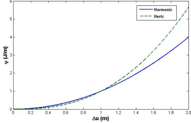
Figure 3: Comparing  $\psi(\Delta u)$  for the Harmonic local potential and Hertz potential.
