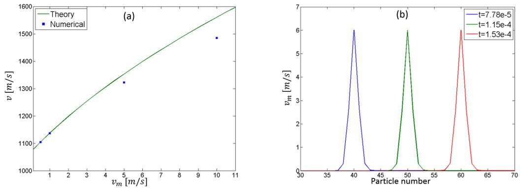
Figure 7: For the weakly nonlinear system, plot (a) shows the propagation velocity  $v$  of solitary waves at different front velocities  $v_m$ . Plot (b) shows  $v_m$  in the chain at different time. Both in the circumstance  $\hat{J} = 0.07$ .
