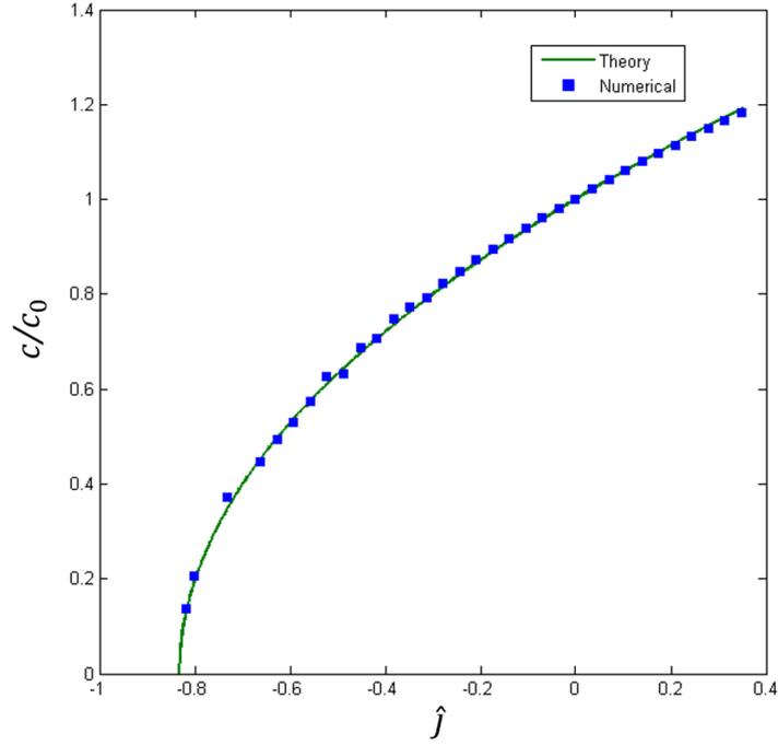
Figure 4: The ratio of wave propagation velocity  $c/c_0$  vs different values of the long-range parameter  $\hat{J}$  in harmonic system, where the initial velocity of the strikers are  $v_i = \pm 5m/s$ .
