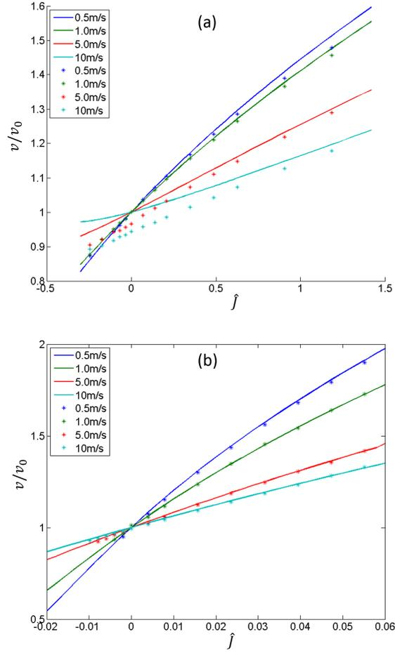
Figure 6: The ratio of wave propagation velocity  $v/v_0$  vs different values of the long-range parameter  $\hat{J}$  in two different systems. Solid lines and discrete asterisks represent theoretical and numerical results respectively. Plot (a) shows the weakly nonlinear system and plot (b) shows the strongly nonlinear system. Different curves correspond to waves propagating at different wave front velocities  $v_m$  in both cases.
