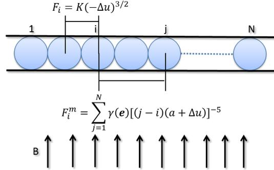
Figure 2: Ferromagnetic granular system under uniform magnetic field
