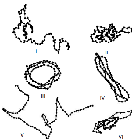
Figure 6. Typical conformations of a 100-segment homopolymer generated by Monte Carlo simulations[26]
