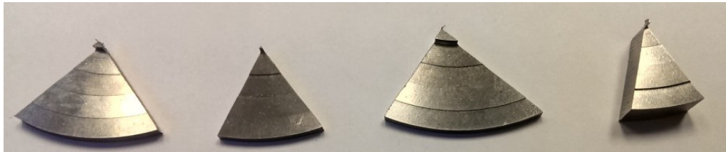
Figure 2.6 IN100 specimens before preparation for grain size measurements.
