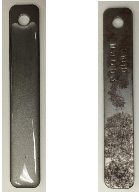
Figure 8 Comparison of the coated side (a) and the uncoated side (b) and stored inside plastic container for 6 months
