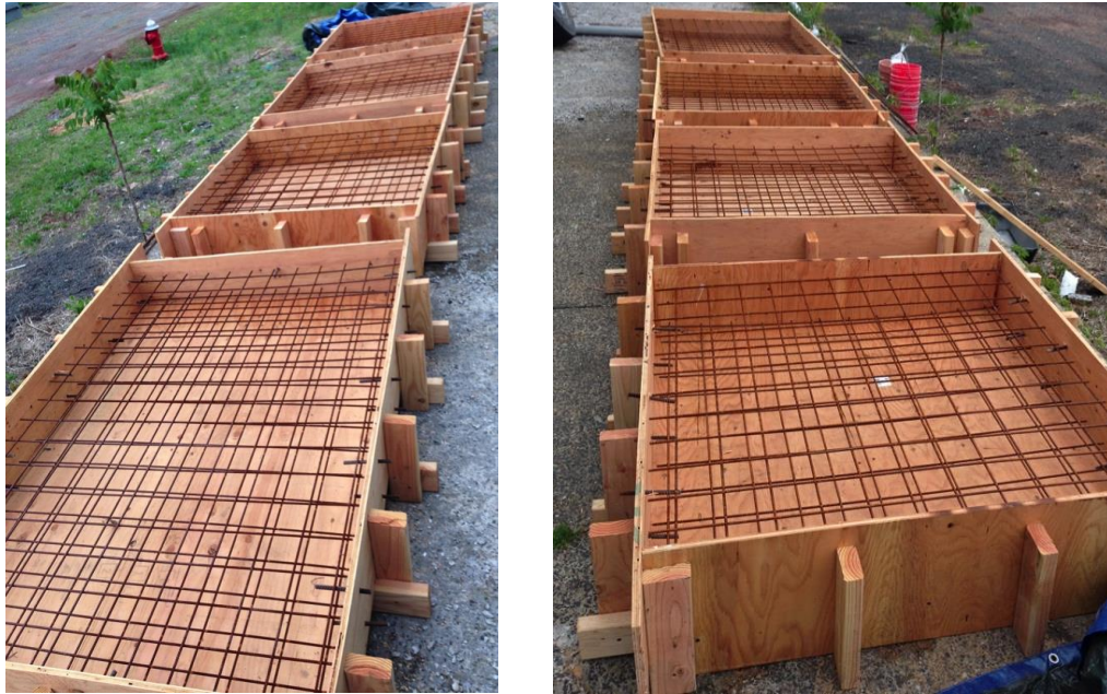
Figure 7.2 Plywood molds for validation specimens
