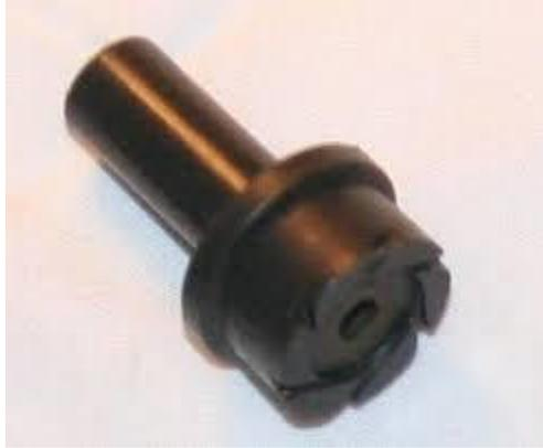
enter the body in a smooth tangential motion in order to form a vortex. It is interchangeable and it also regulates the volume of compressed gas so that flow rate and temperature ranges can be controlled.
