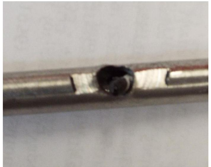
**Figure 22. Suspension of thermistor through a SS tube**
