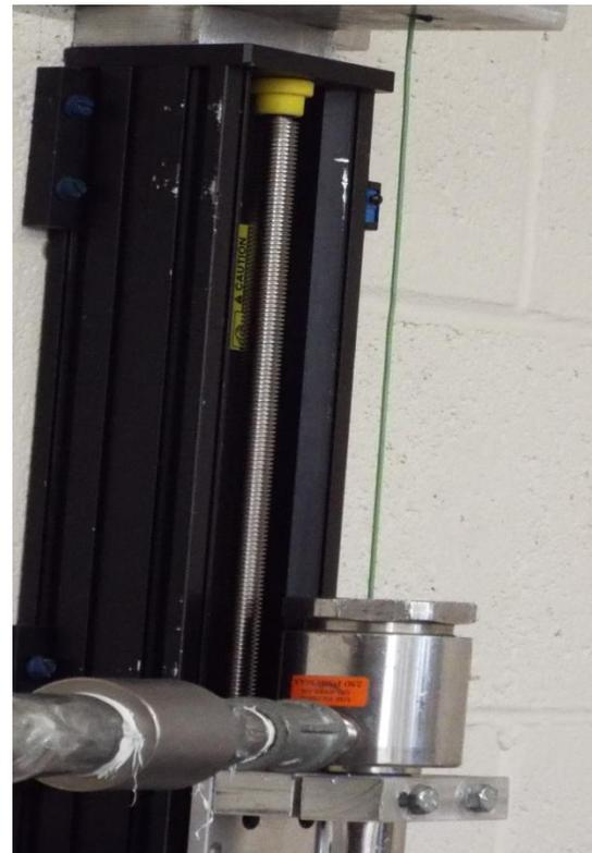
Figure 23. Measurement of vibrations induced in the wire
