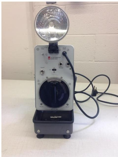
**Figure 31. Stroboscope**
