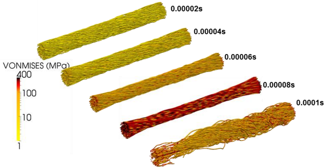
Figure 3.14 Von Mises plots of yarn at varying times of the analysis. As the analysis progresses (top to bottom) stress points grow until fiber breakage and unwinding.
