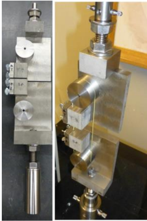
Figure 5.1 The AMSL grip design attached to the Instron tensile machine. The yarn is gripped on top then passes through 180° rotation in the hemispherical grooves on the top cylinder. It passes through another 180 deg. rotation on the bottom cylinder and is gripped on the bottom. The minimum gauge length that can be tested by this design is 10 inches.
