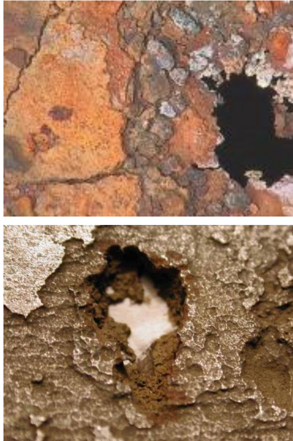
Figure 1.1: LNG pipeline failure due to corrosion
