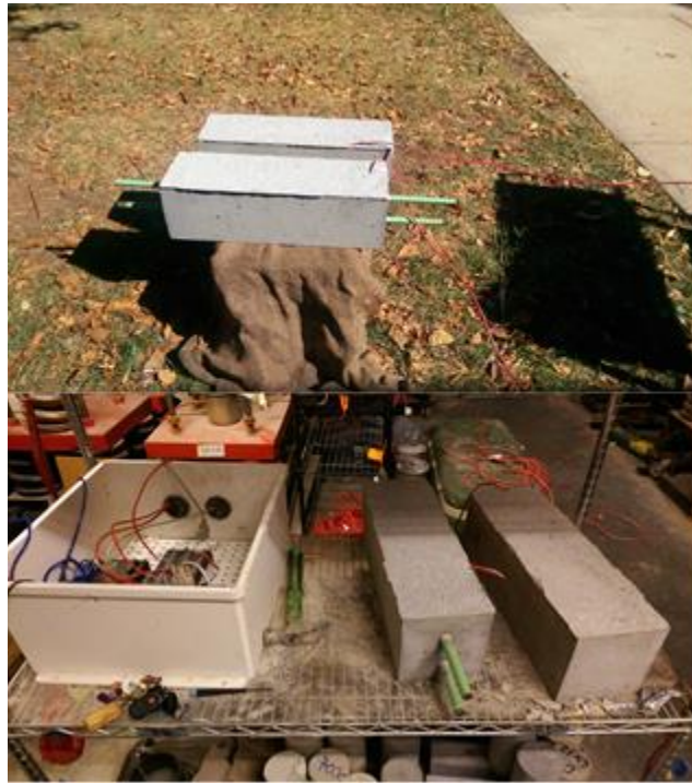
Figure 7: Concrete samples for experimental setup 4 stored in chamber and outdoors
