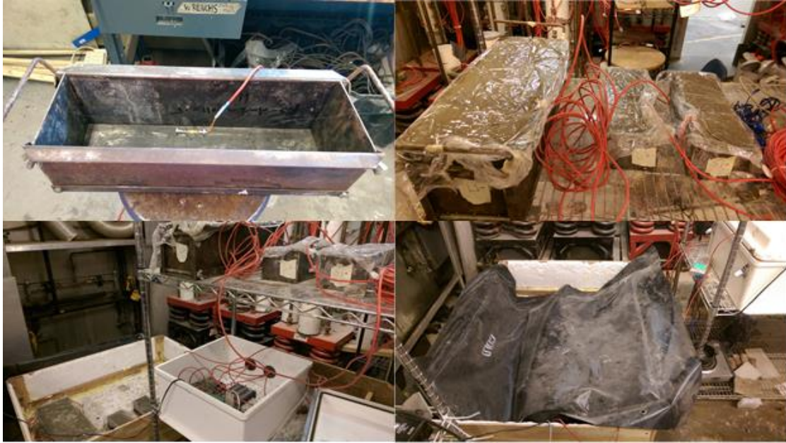
Figure 5: a) Free shrinkage prism mold with embedded VWSG b) Concrete prisms stored in environmental chamber c) Concrete prisms connected to datalogger d) Concrete prism stored under heat blanket (top left to bottom right)
