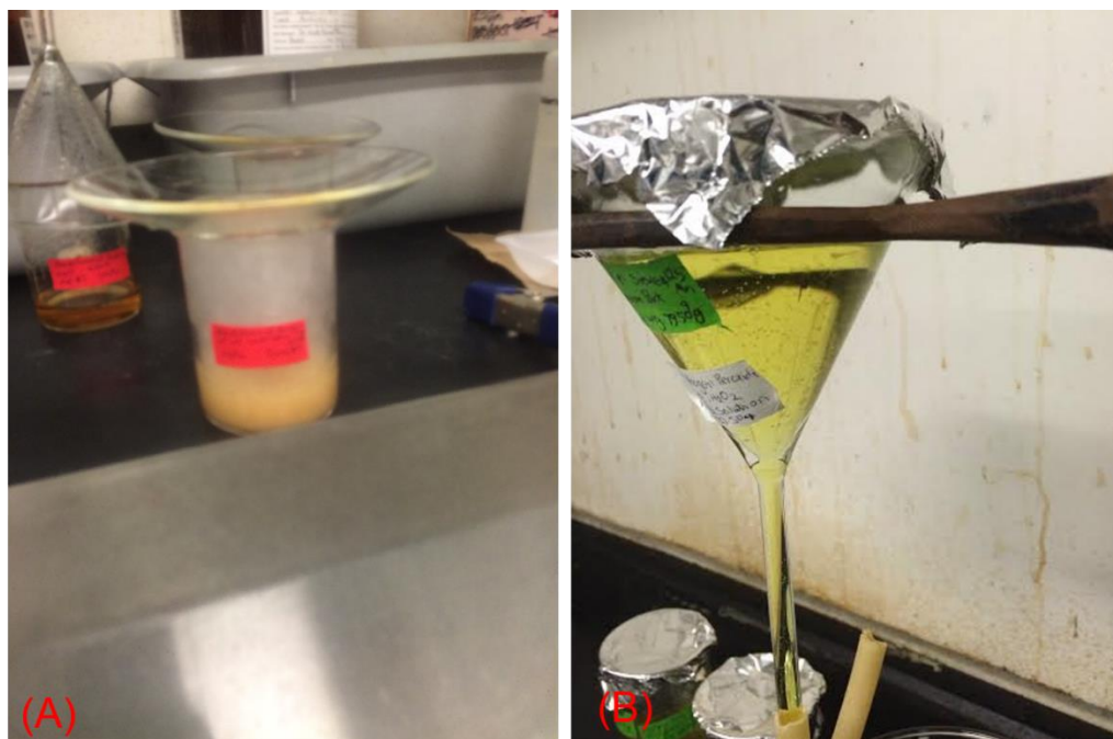
Figure 3-Experimental Steps (A) Wet Peroxide Oxidation of Organic Material, (B) Density Separation of microplastic particles
