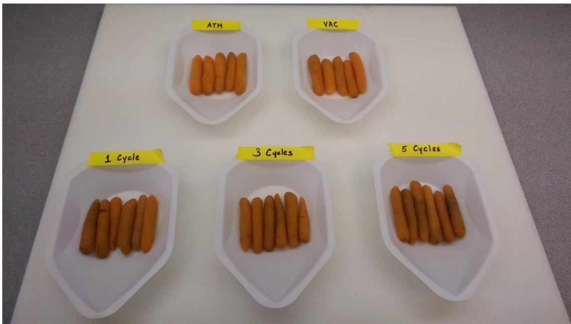
Figure 35. Baby carrots after calcium infusion under different conditions
