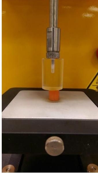
Figure 19a. 1 cm long baby carrot cylinder before compression
