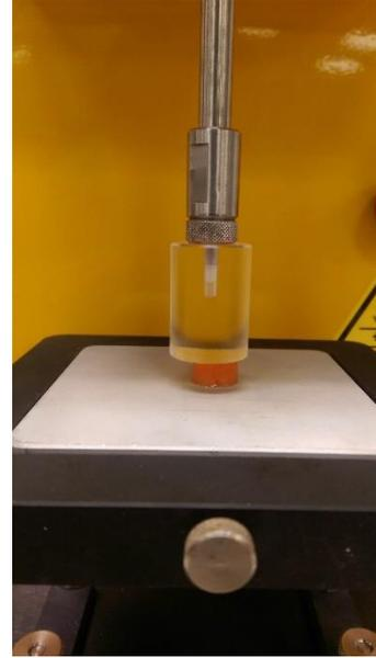
Figure 19b. Baby carrot cylinder after compression
