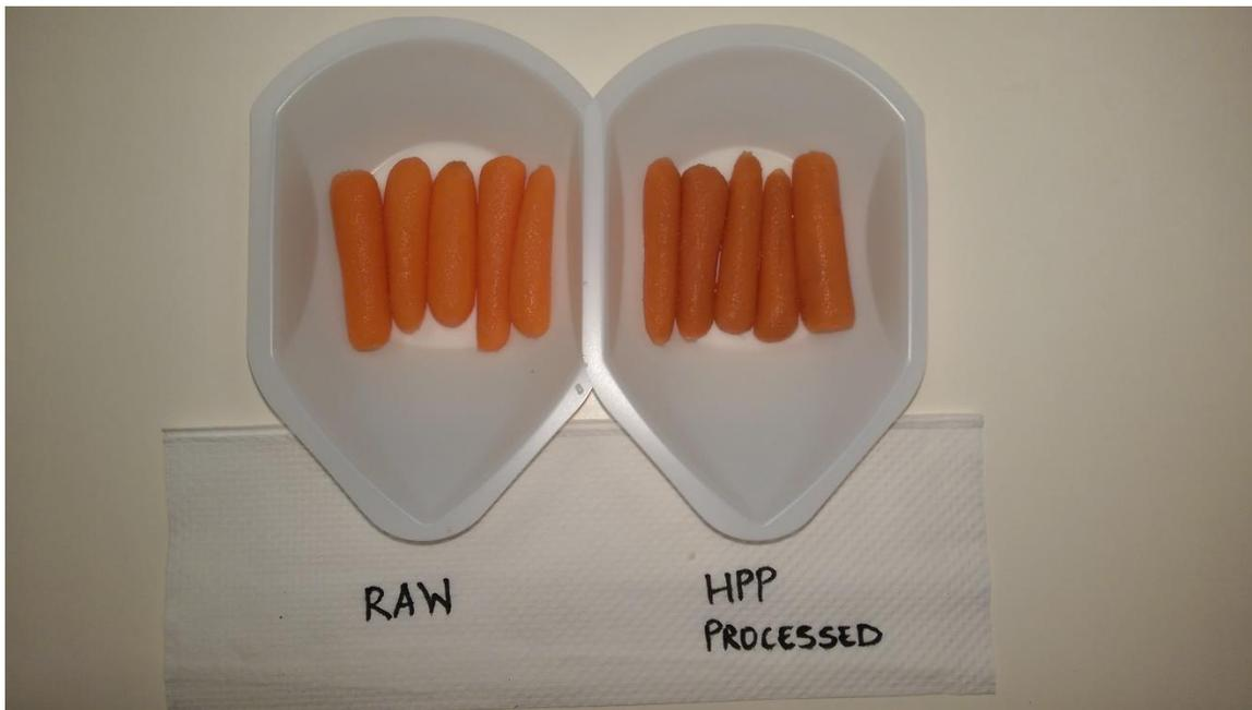
Figure 26. Baby carrots before and after high pressure-calcium infusion. The processed baby carrots in this figure were processed at the center point (350 MPa, 10 min, 6 % CLG solution concentration).
