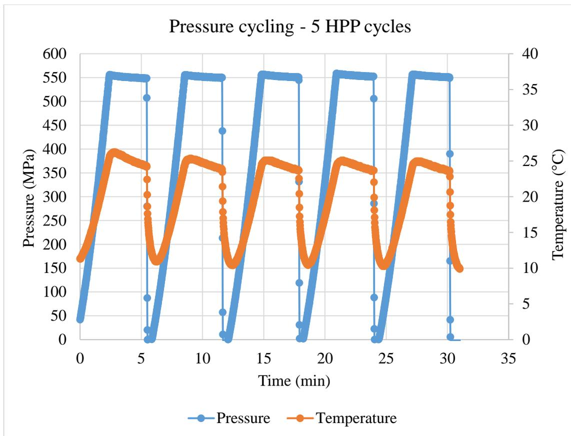
Figure 11c. Pressure cycling – 5 cycles, as recorded in the LabVIEW™ software.
