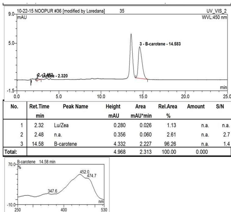
Figure 16. HPLC chromatogram of beta-carotene analysis
