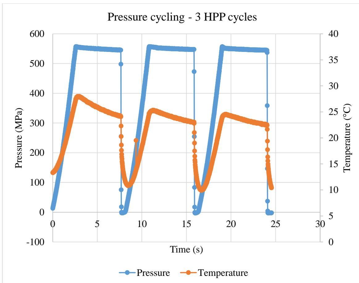
Figure 11b. Pressure cycling – 3 cycles, as recorded in the LabVIEW™ software.
