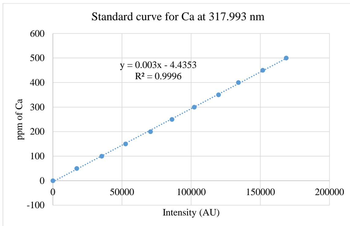
Figure 14. Standard curve for estimation of calcium at 317.993 nm
