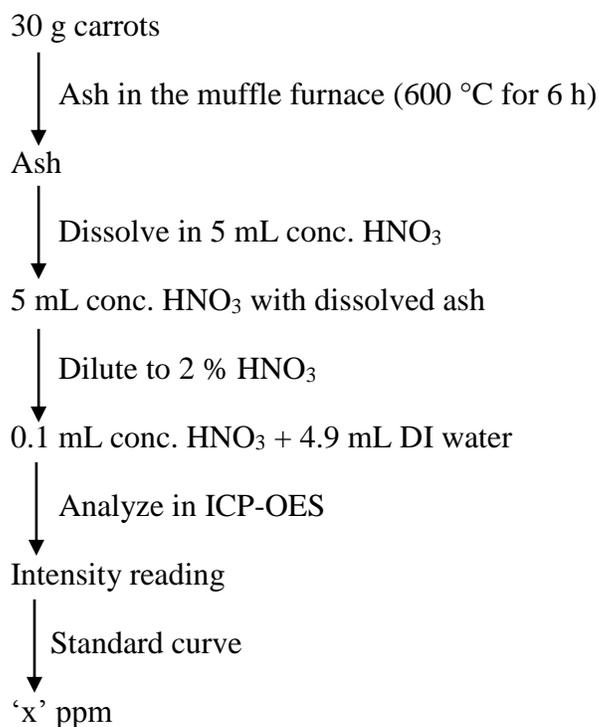
Figure 15. Flow chart for sample preparation for calcium analysis
