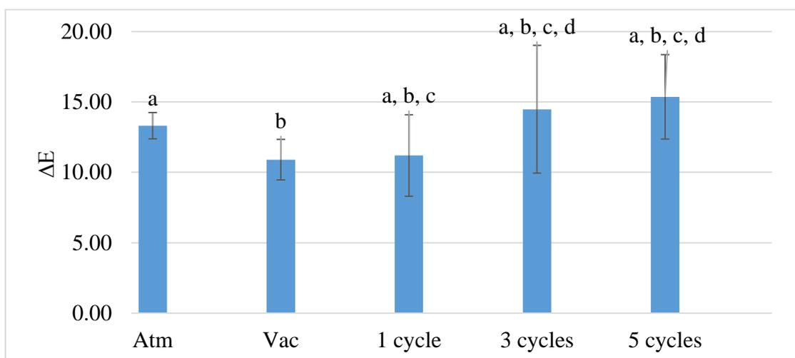
Figure 34. Effect of pressure cycling on the change in color of the high pressure processed-calcium infused baby carrots and comparison to controls\*
