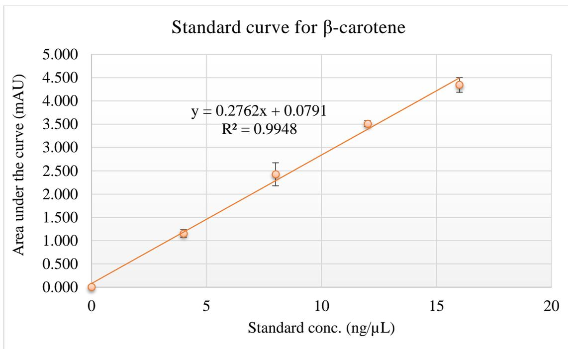
Figure 17. Standard curve for estimation of beta-carotene in baby carrots
