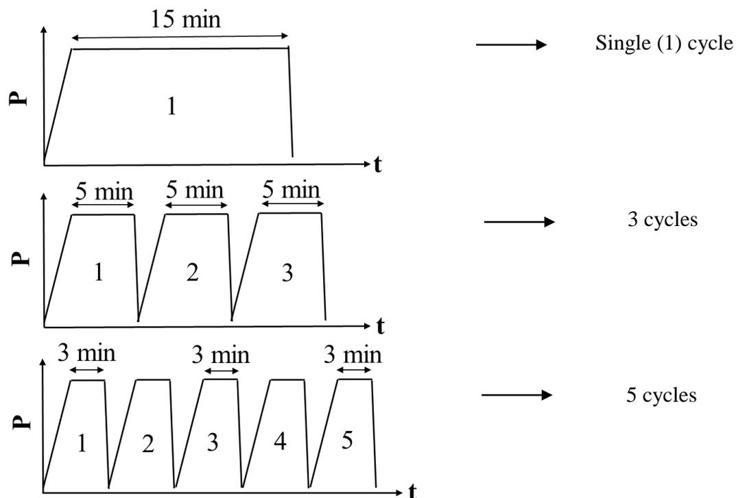
Figure 9. Pressure cycling and hold time during each cycle.
