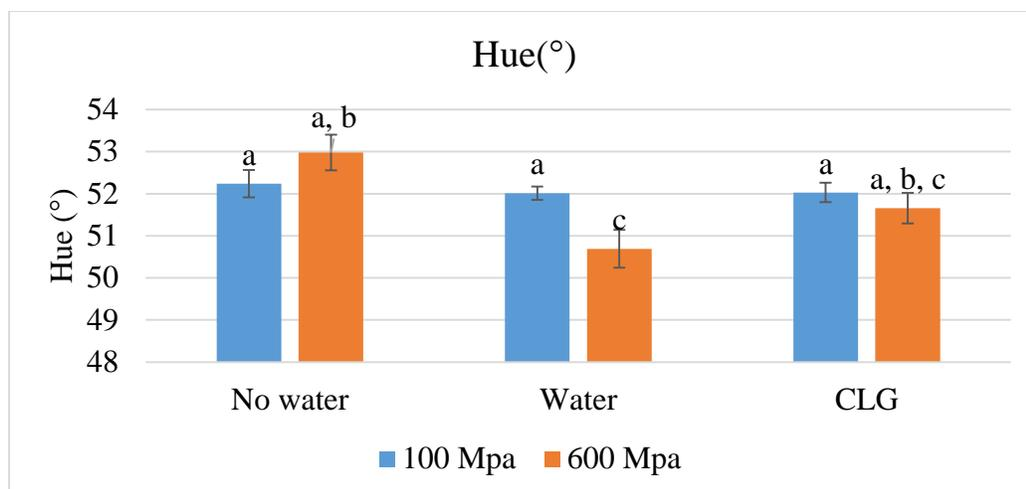
Figure 36c. Effect of calcium infusion and extent of high pressure on the Hue (°) of the processed baby carrots\*
