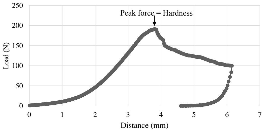
Figure 20. Texture analysis graph for compression of a baby carrot cylinder by 50 % (Test speed = 1 mm/s)
