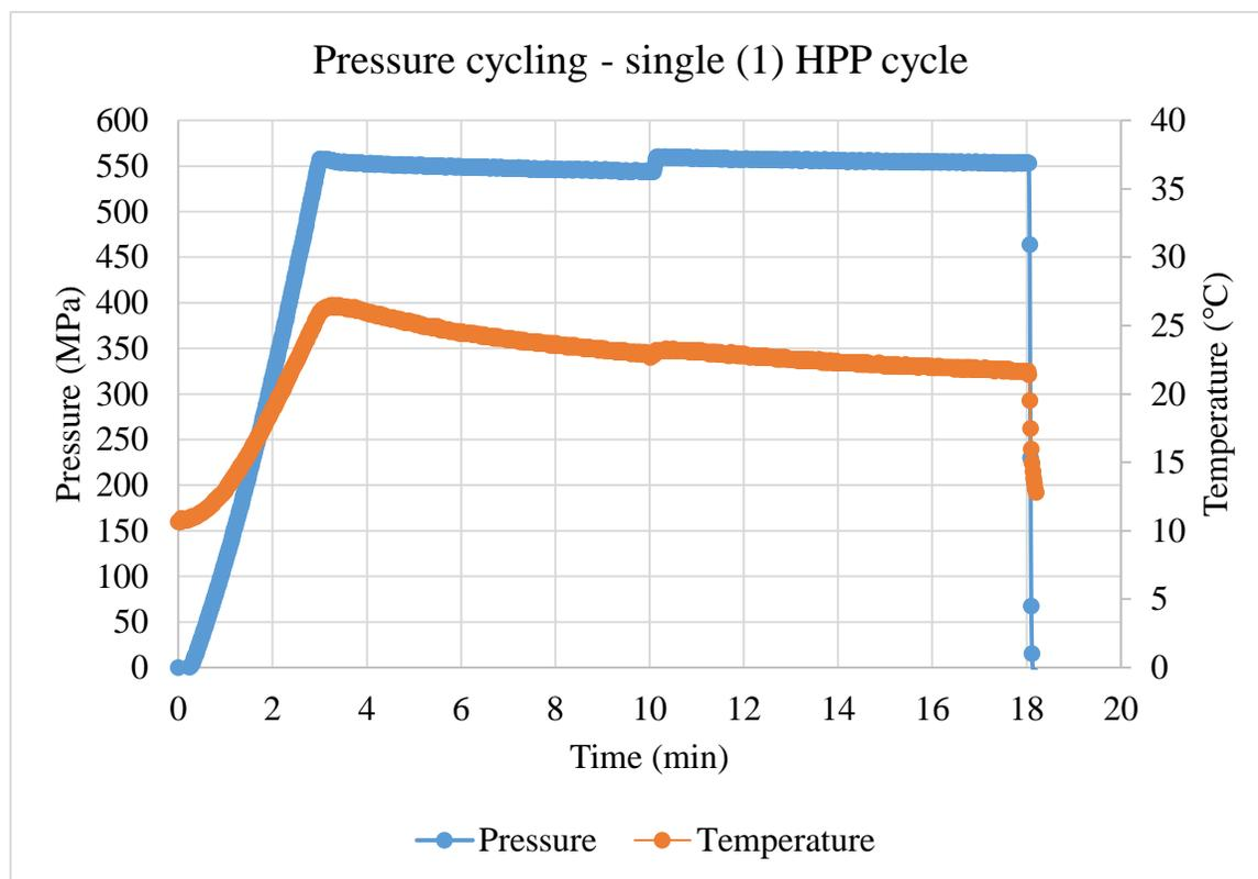
Figure 11a. Single pressure cycle as recorded in the LabVIEW™ software.
