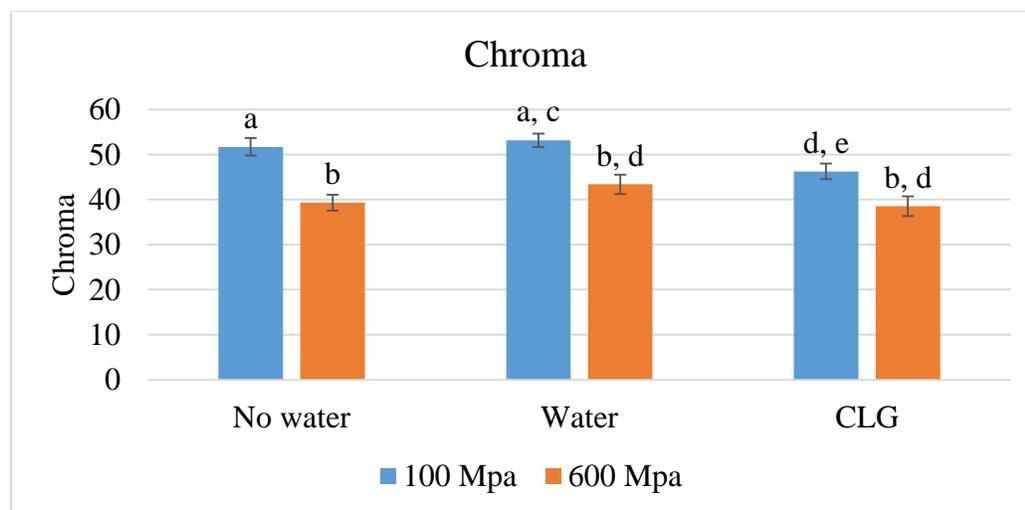
Figure 36b. Effect of calcium infusion and extent of high pressure on the Chroma of the processed baby carrots\*
