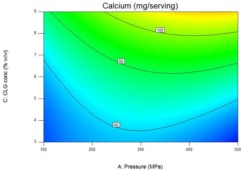
Figure 22. Effect of pressure-CLG solution concentration interaction on the infusion of calcium at a constant processing time of 10 min.
