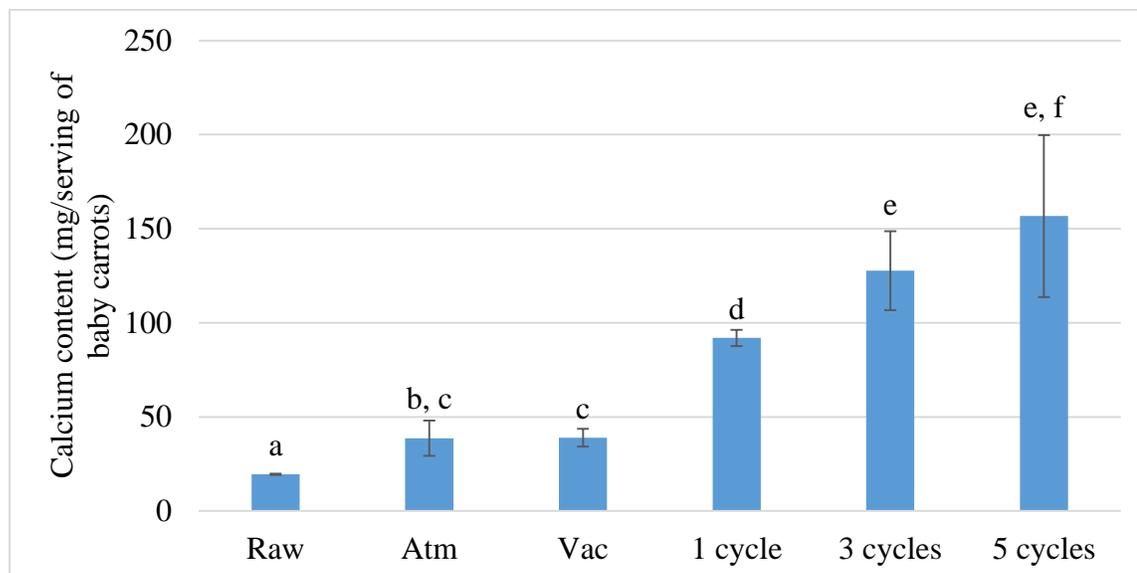
Figure 27. Calcium infused during pressure cycling and comparison to controls\*
