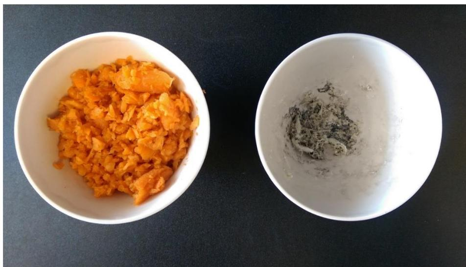
Figure 12. Carrot samples before (left) and after (right) ashing.
