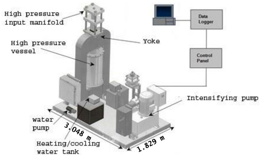
Figure 3. Schematic representation of high pressure processing unit at the Department of Food Science, Rutgers University.
