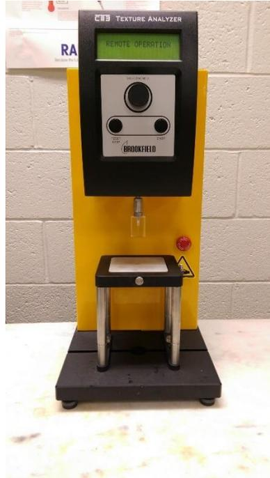
Figure 18. CT3 Brookfield Texture Analyzer used for texture analysis of baby carrots
