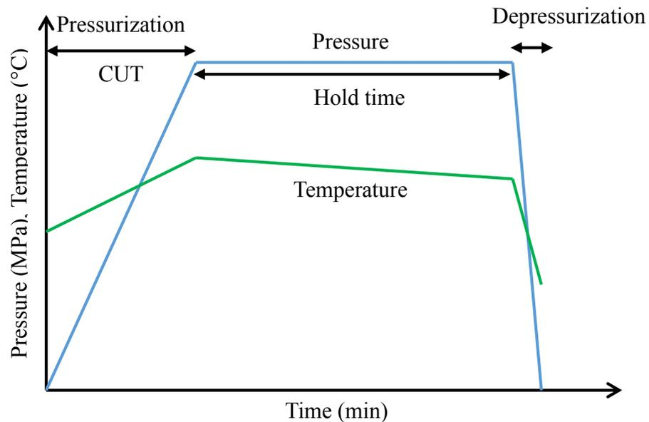
Figure 4. Variation of pressure (MPa) and temperature (°C) during the HPP cycle
