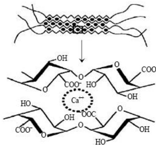
Figure 6b. Egg-box model of calcium and pectin complex
