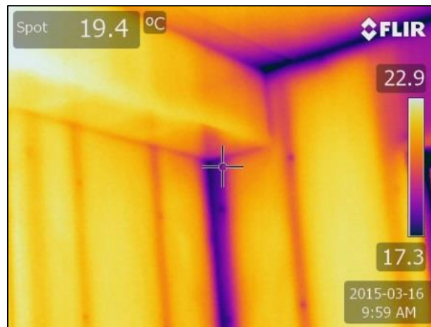
Figure 6: Thermography of interior wall surface with thermal bridge in winter
