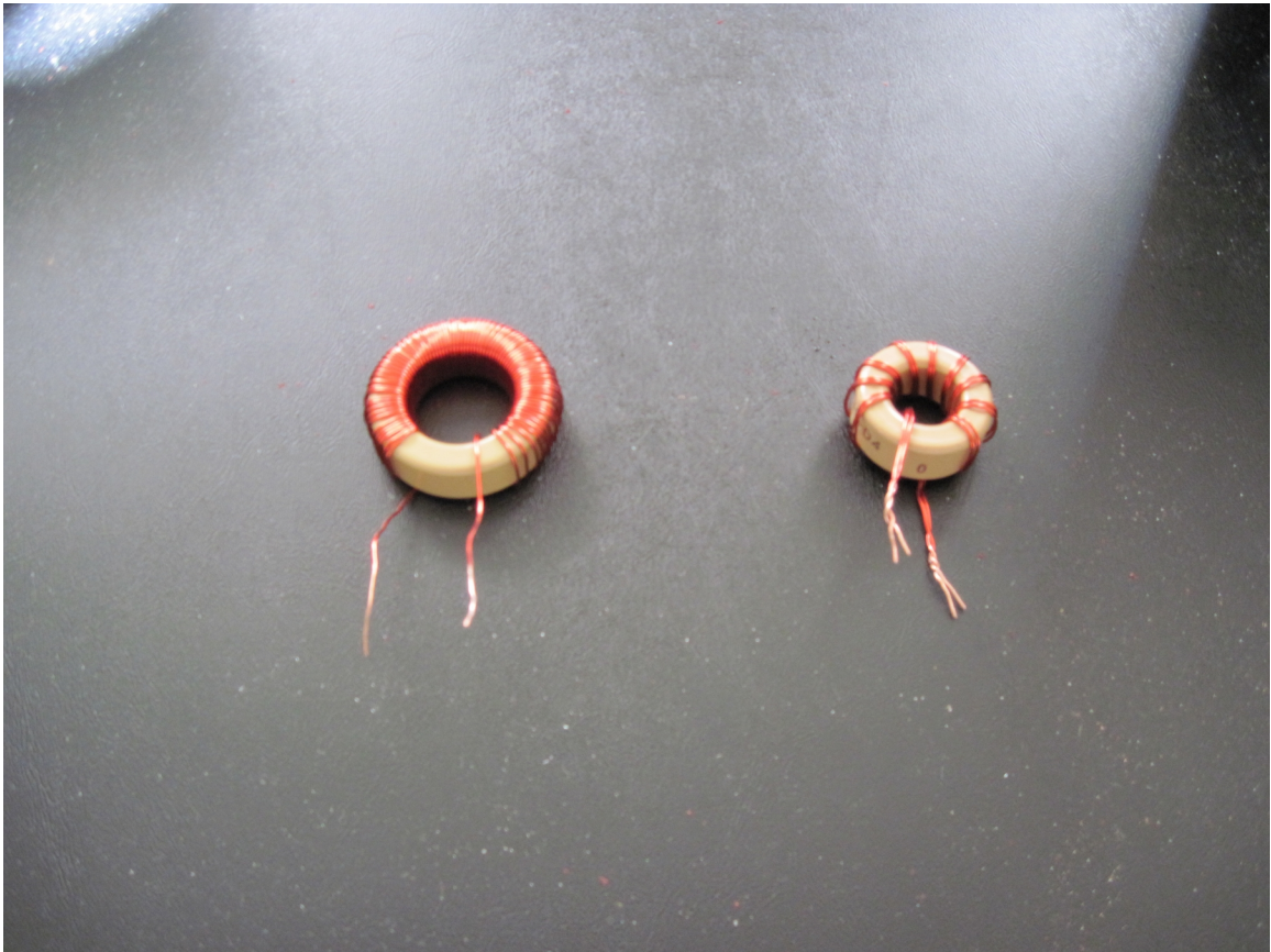
Fig. 4.26. Hand wound inductors L_1 and L_2 .
