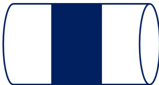
Figure 3-2: Initial loading condition of the cylinder. The middle 1/3 rd of the cylinder is loaded with dyed material. 1/3 rd sections on the two ends are loaded with undyed material. A fill volume of 35% was kept constant for all materials.
