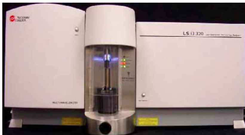
Figure 2-1: Beckman Coulter LS 13 320 laser diffraction based particle size analyzer. The tornado system fluidizes particles to measure the size of individual grains
