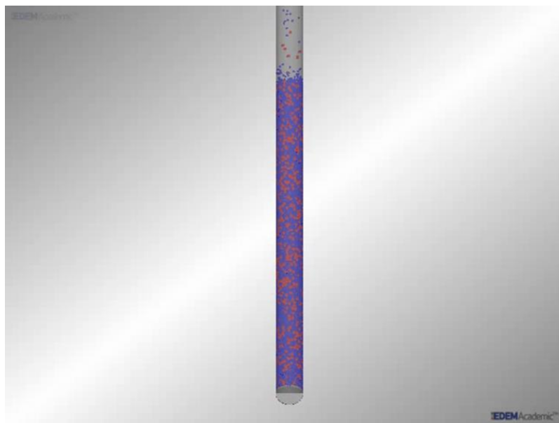
Figure 7-3: A screen shot of a simulation modeling dense granular transport in a vertical bed. The rotation speed of the valve is tuned to match the rate of material addition to the simulation
