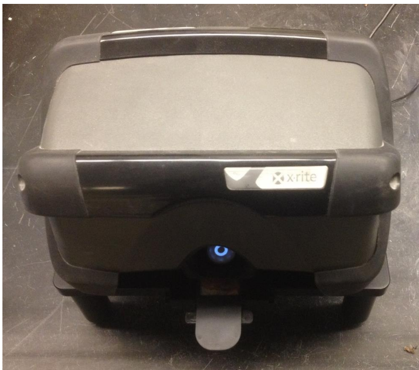
Figure 2-5: X-Rite VS-450 colorimeter. The colorimeter shines visible light on the sample and measures the consequent reflectance
