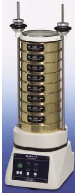
Figure 2-3: Endocotts sieve shaker. The shaking ensures percolation of the grains through the sieves until they encounter perforations smaller than, typically, their second largest dimension.
