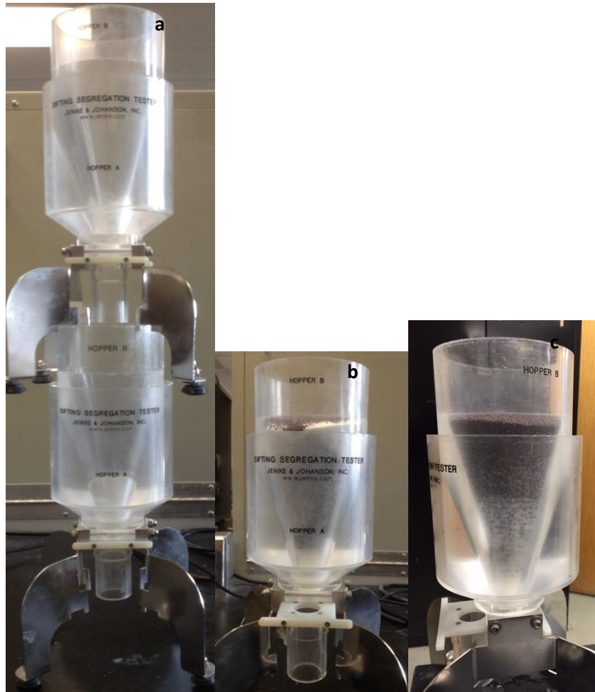
Figure 4-1: (a) Jenike segregation hoppers mounted as they would be during testing; (b) mixture of sugar and mustard seeds after they are loaded in the hopper, ready for testing; (c) mixture of sugar and mustard seeds after 10 hopper cycles
