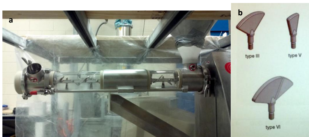
Figure 4-3: (a) Glatt GCG-70 continuous tubular blender with its (b) blade types. Type III blades were used during the course of the entire study.
