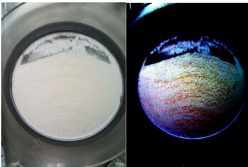
Figure 7-2: Formation of axial bands in during transport of material in a vertical packed bed. The axial bands can manifest in the final product leading to content non-uniformity.
