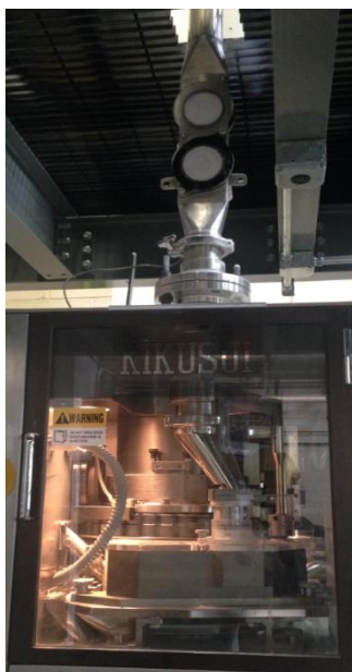
Figure 4-1: Pilot- scale compaction setup. Post- blending, the blend was dispensed to the tablet press through a chute. 6 tablets were collected every minute for the entire duration of compaction.
