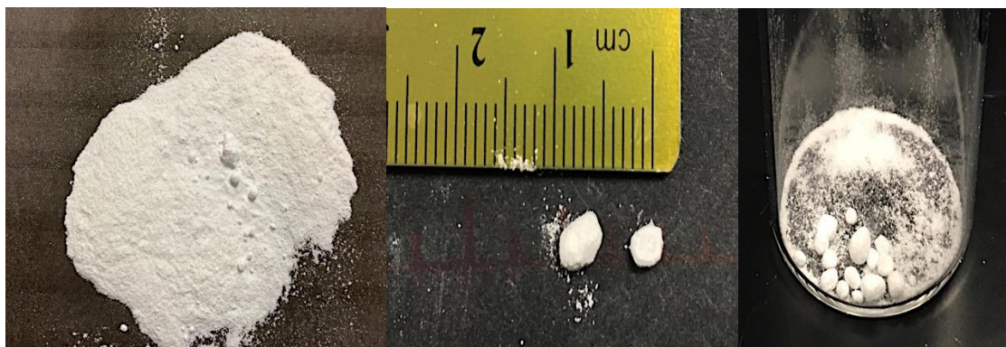
Figure 5-3: Agglomerates observed in thief samples, agglomerate size ranging up to 5 mm.
