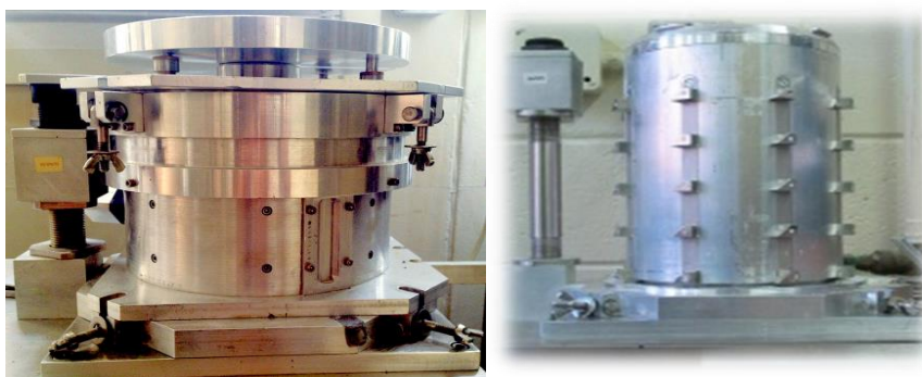
Figure 2.3: Shearing device used to impart uniform shear on blends. Inside cylinder of the Couette shear cell assembly with the baffles (right) The blend is poured in the annular region and the cylinders move relative to each other imparting the shear
