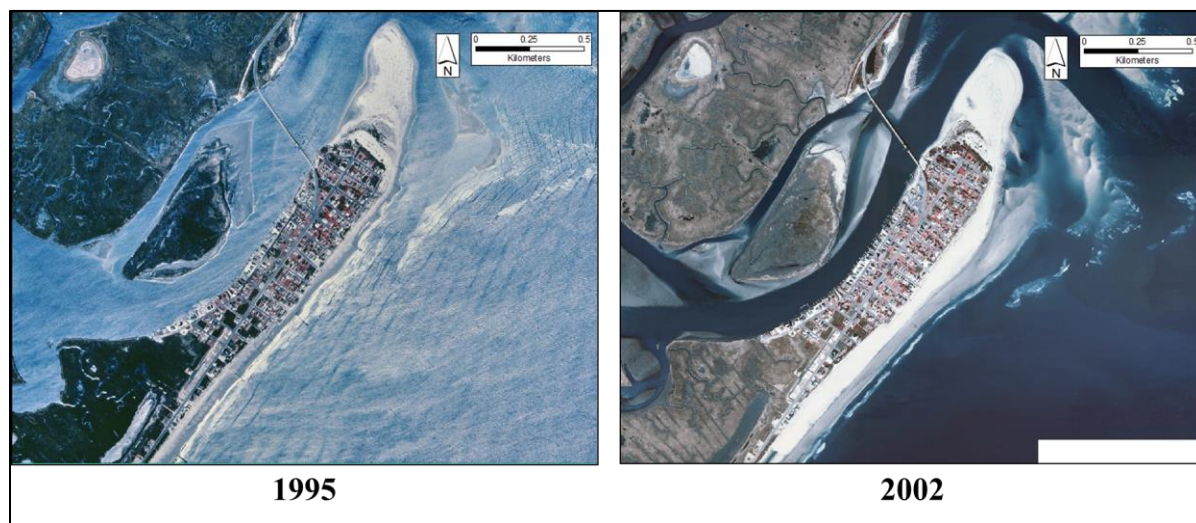
Figure 32. Aerial images of the northern end of Ludlam Island from 1995 (left) and 2002(right) showing how shore protection structures such as groins visible in the earlier photograph are not visible in the later photograph, and thus not delineated for the study.
