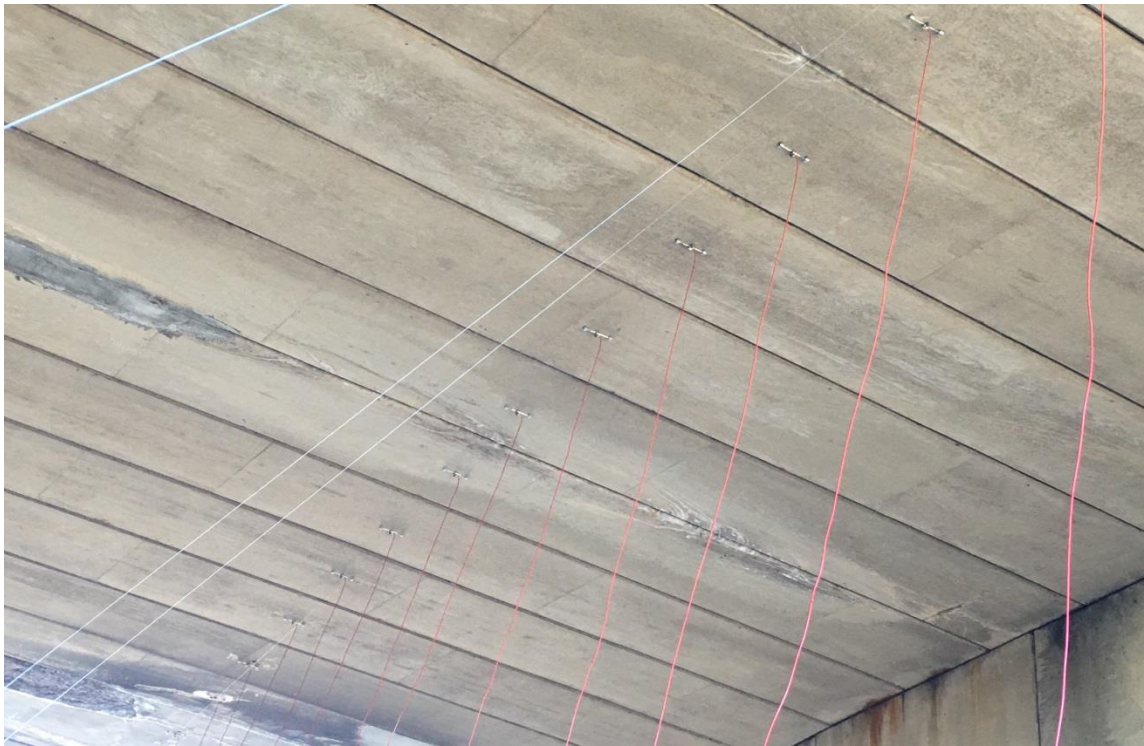
Figure 4.16 - Installed 4000 Vibrating wire strain Gauges and PT 8510
