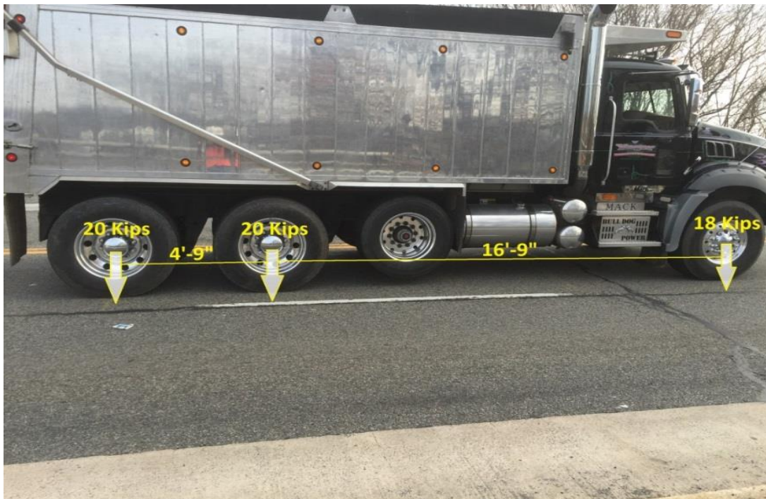
Figure 4.17 - The weights and distances for the load vehicle
