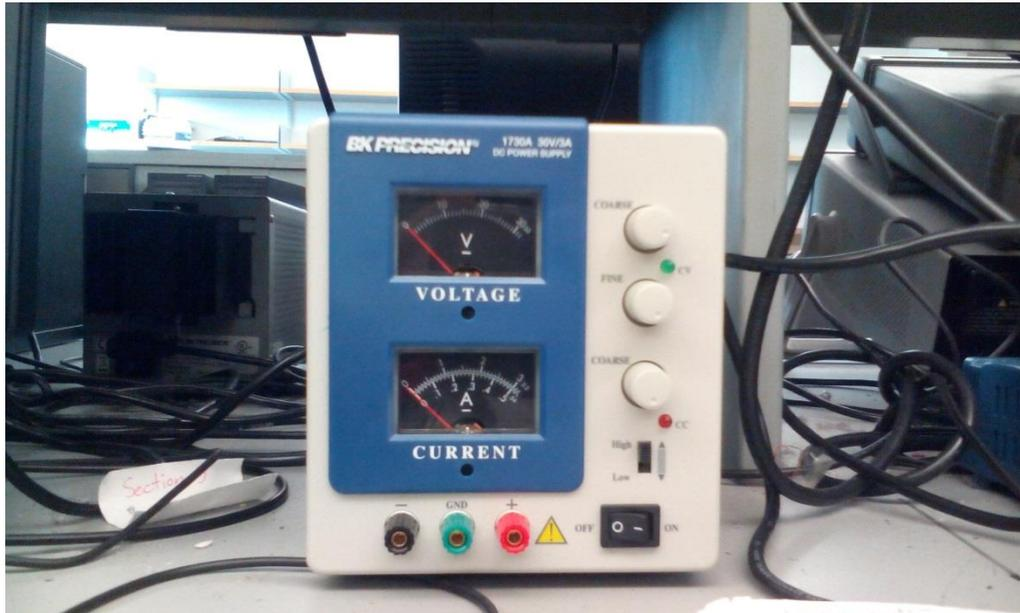
Fig 3.2: Adjustable DC power supply
