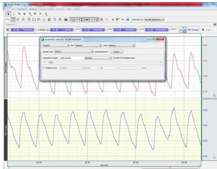
Fig 3.13: BSL settings-Sampling rate and acquisition length
