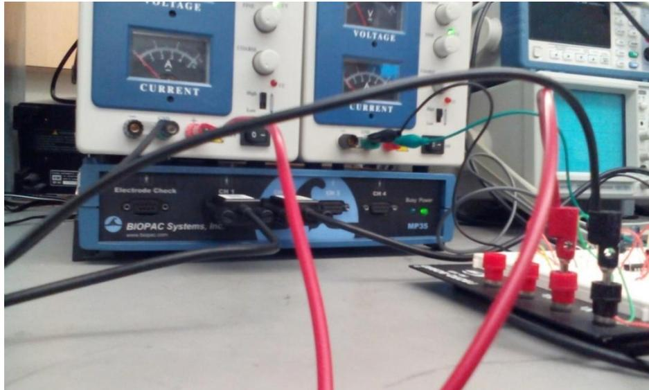
Fig 3.8: Biopac MP36 data acquisition port and its connection with the Dual PPG circuits
