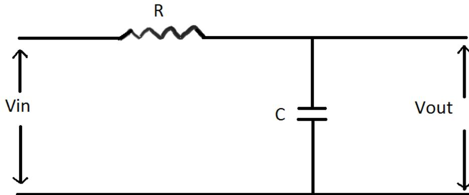
Fig 3.5: Schematic diagram for RC low pass filter
