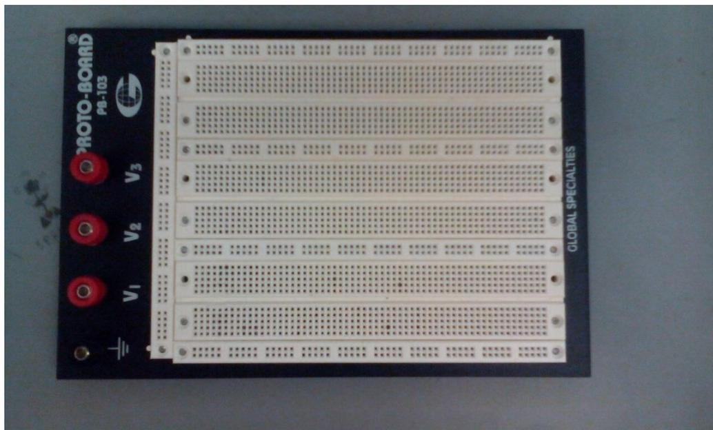
Fig 3.1: Electrical breadboard
