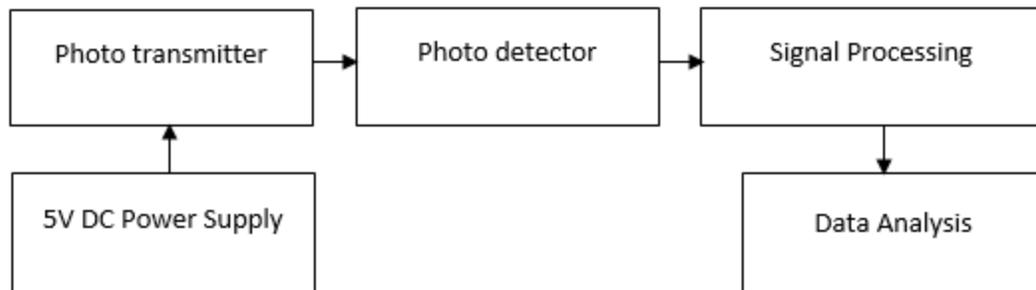
Fig 1.3: General schematic diagram of a photoplethysmographic recording system
