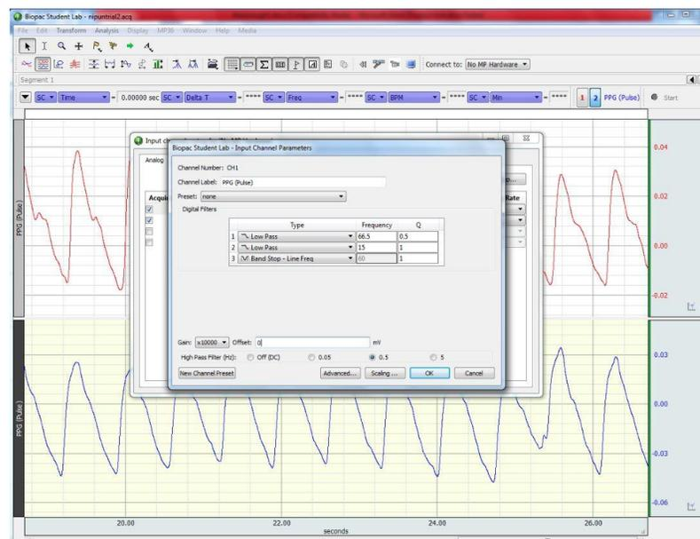
Fig 3.11: BSL settings-Filter and gain selection
