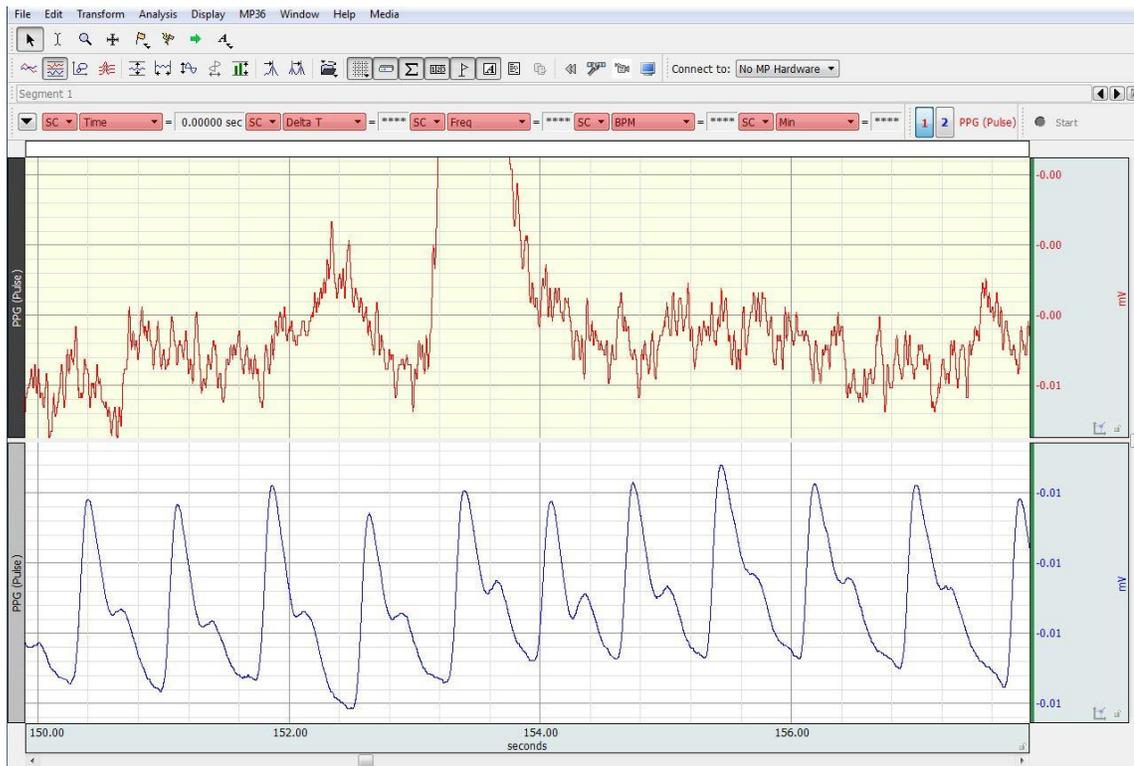
Fig 5.1: Limitation of design instability and resultant noise in acquired PPG-Red: Noisy brachial artery PPG and Blue: Stable finger PPG
