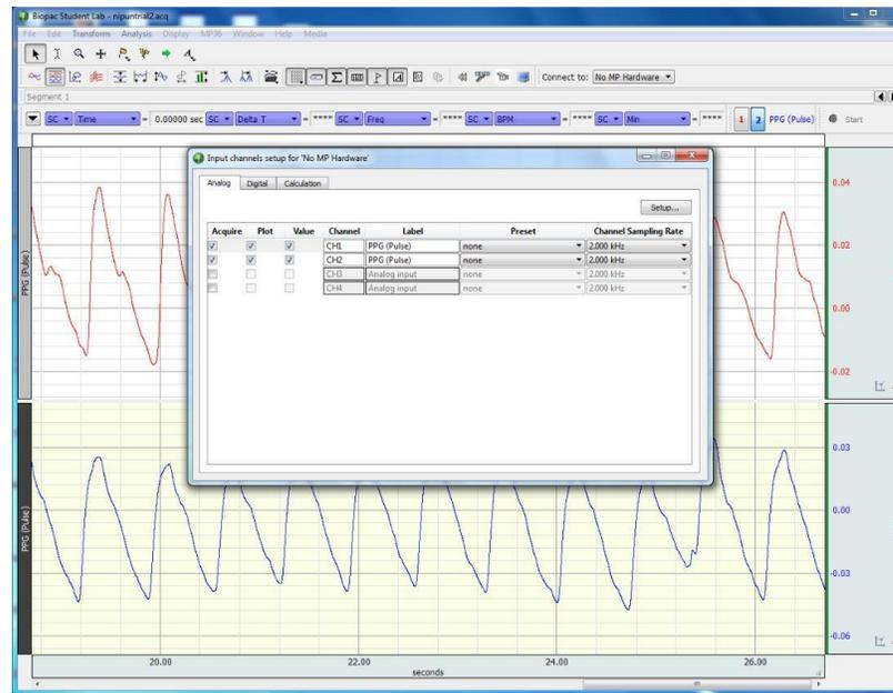
Fig 3.10: BSL settings-Channel selection and sampling rate
