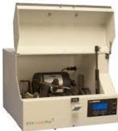
Figure 43. Spex mill used to develop mechanical mixtures of carbon and boron carbide.
