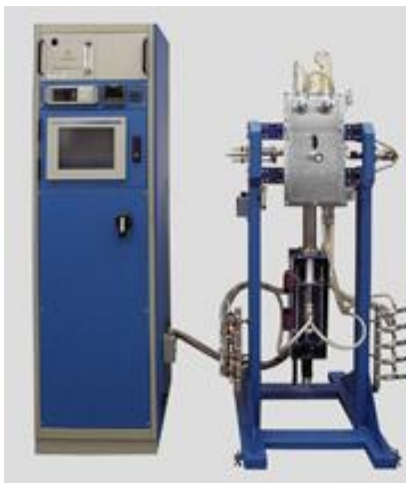
Figure 64. Oxy-gon High Temperature Vacuum Furnace System used to hot press mixtures of amorphous boron and boron carbide.
