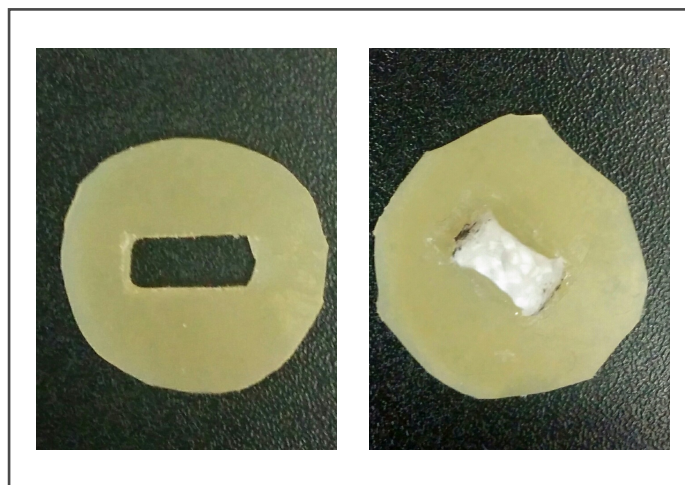
Figure 3: (a) Non-porous plastic base, (b) Scaffold placed over the opening.
