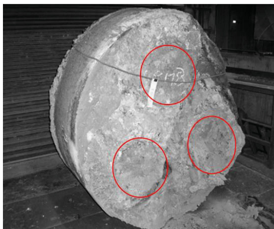
Figure 8. An ingot of boron carbide synthesized using the electric arc furnace. Circles indicate regions of reacted boron carbide (Courtesy of Washington Mills, Niagara Falls, NY).
