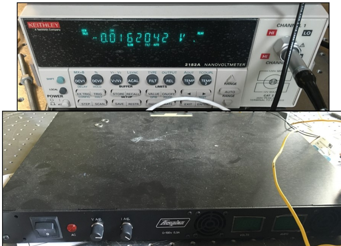
Figure 5–36: Nanovoltmeter (top) and Power Supply (bottom) used for Seebeck Coefficient Measurements
