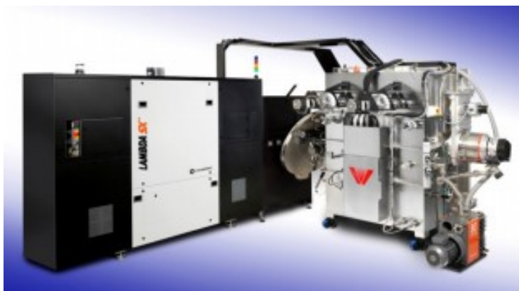
Figure 2–9: Commercial reel-to-reel PLD tool capable of depositing films over 1 cm wide by 1 km long with a total effective area of 10 m 2 (reproduced with caption from [21])
