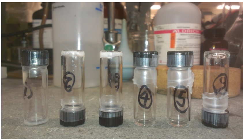
Figure 3S8-1. Appearance of Six PA Samples at Various Solution pHs. Vial #1-3: 80 mM \text{C}_{12}\text{Ala-Phe} at pH 6.7 (#1, cloudy solution), pH 6.0 (#2, gel) and pH 5.5 (#3, gel). Vial #4-6: 100 mM of \text{C}_{12}\text{Gly-Glu} at pH 6.0 (#4, solution), pH 5.0 (#5, solution) and pH 4.5 (#6, gel).
