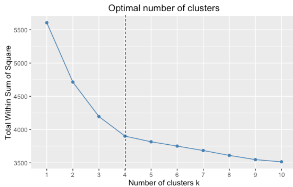
Figure 43 Elbow plot of optimal number of clusters
