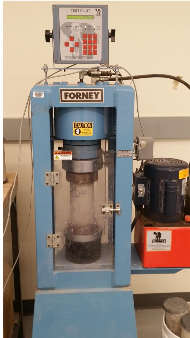
Figure 37: Concrete cylinder in compression machine cage
