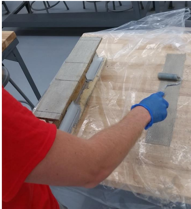
Figure 35: Roller removing excess nano-inorganic composite from basalt fiber
