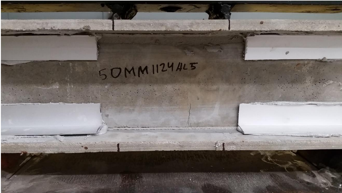
Figure 43: Extent of cracking for first phase of testing
