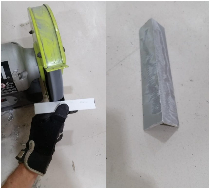
Figure 23: Left (a) Grinding aluminum angle; Right (b) Grinded aluminum angle
