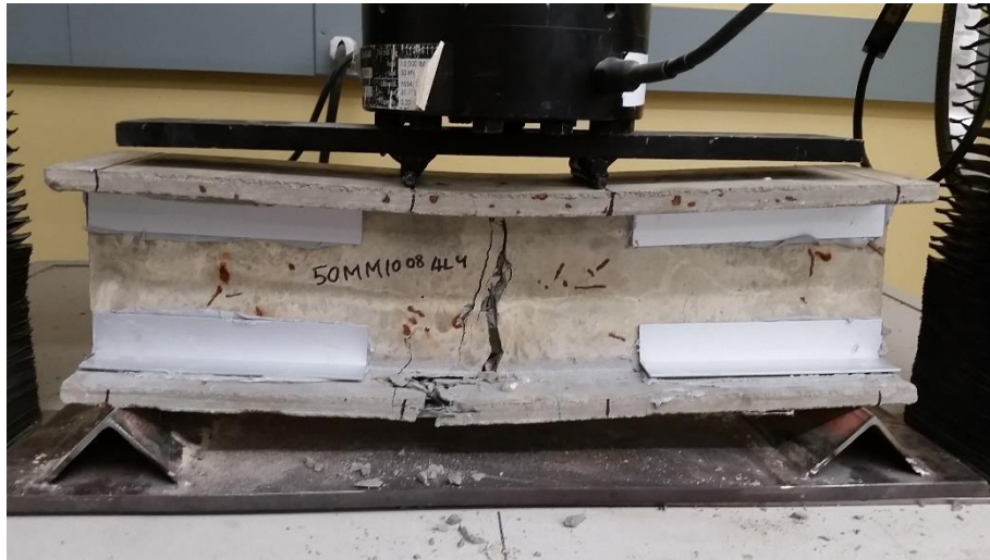
Figure 24: Beams Tested to Failure with External Flexural Reinforcement (a) 6MM-0323-FRP6; (b) 13MM-0317-FRP5; (c) 6&30MM-0323-AL5; (d) 13&50MM-0318-AL4; (e) 30MM-1124-AL6; (f) 50MM-1008-AL4
