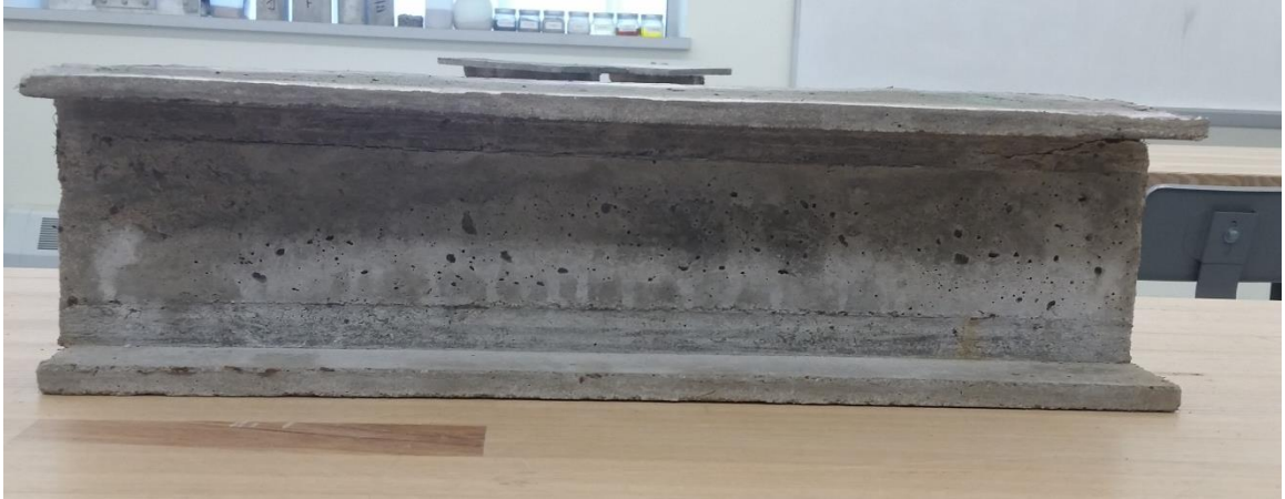
Figure 57: Cracks that occurred during dry curing
