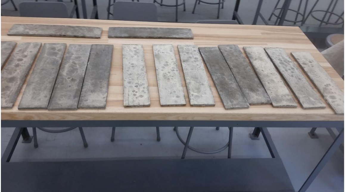
Figure 19: Concrete plate samples in temperature controlled lab environment
