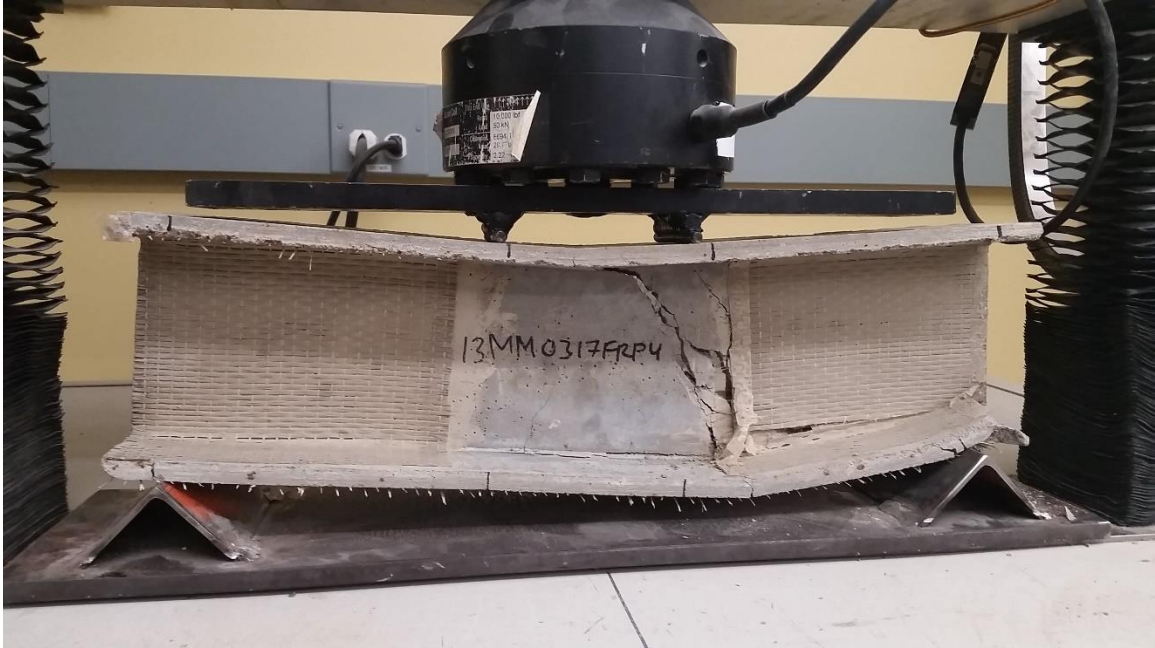
Figure 44: Shear and flexural cracks present in beam during testing
