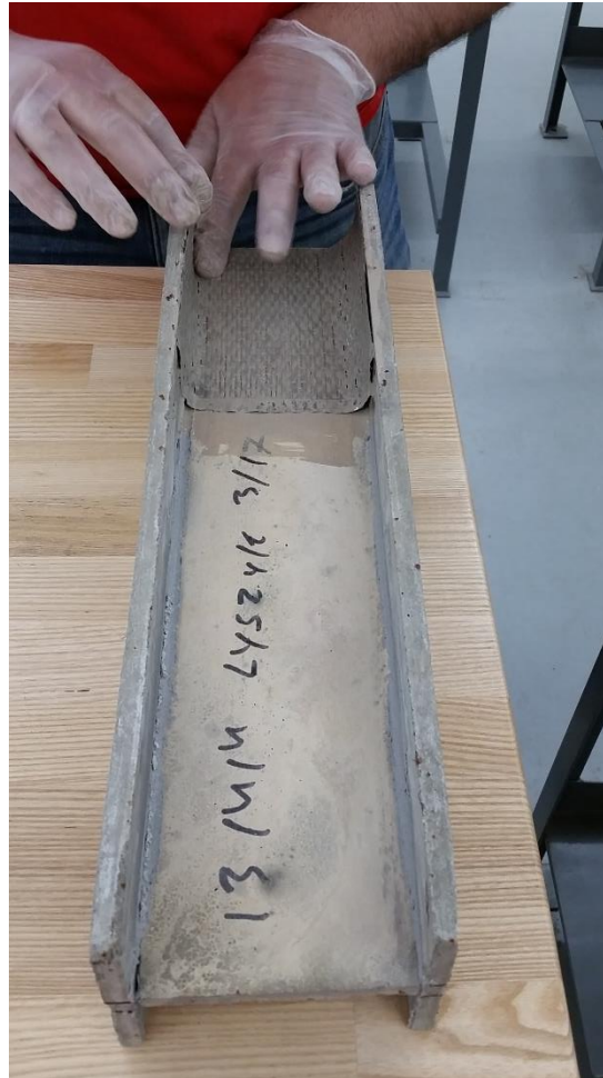
Figure 32: Applying slight downward pressure on basalt fiber
