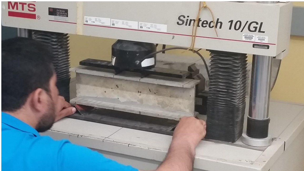
Figure 41: Positioning of beam onto point supports
