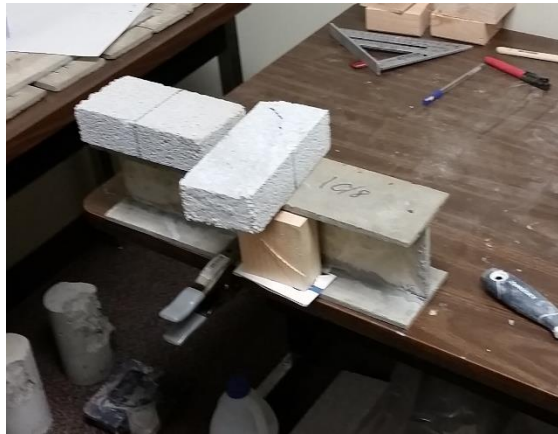
Figure 28: Bricks and wood blocks stabilizing beam configuration
