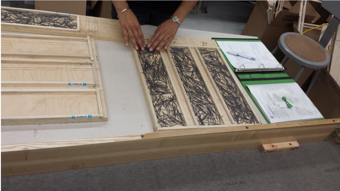
Figure 12: Placing 50 mm hooked end fibers in wooden molds prior to mixing
