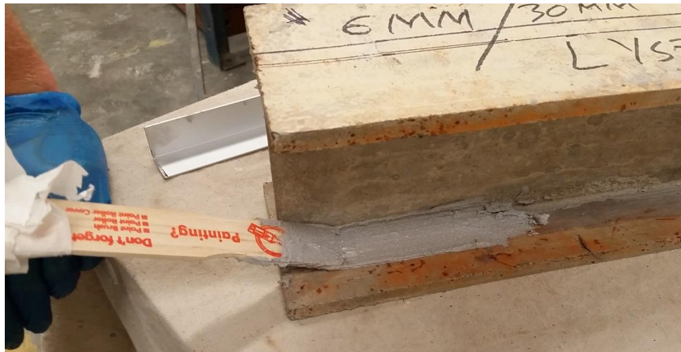
Figure 33: Applying epoxy to flange for aluminum angle attachment
