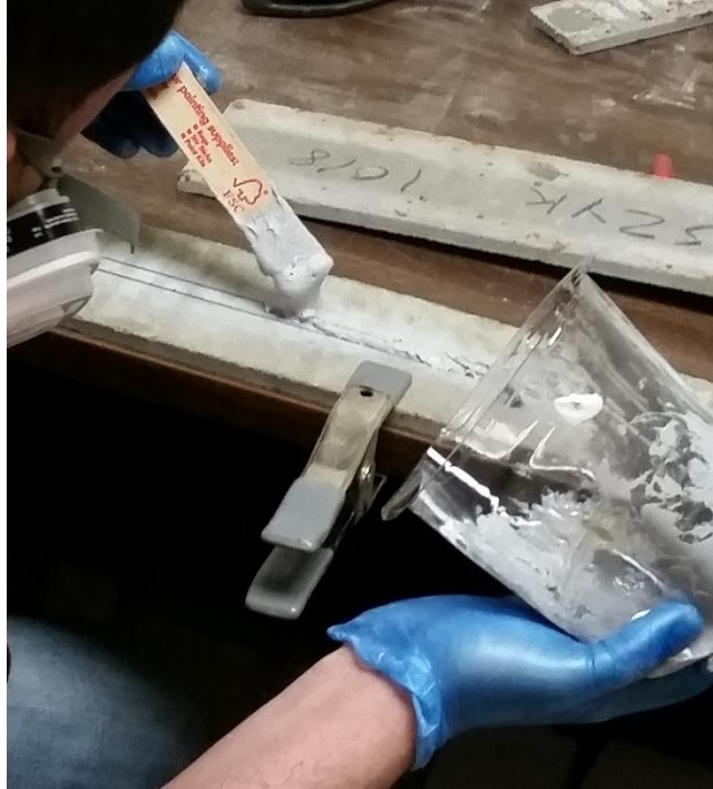
Figure 26: Applying epoxy to concrete plate
