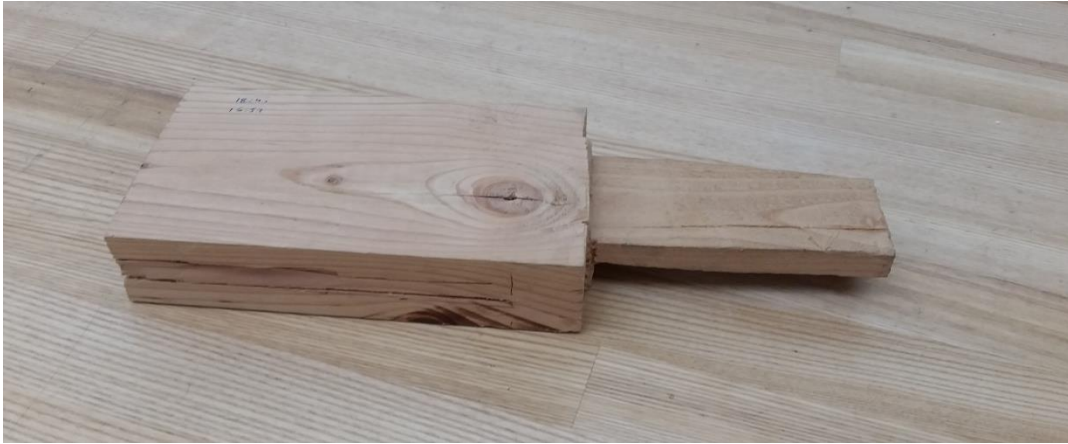
Figure 47: Intermediate grip made out of wood
