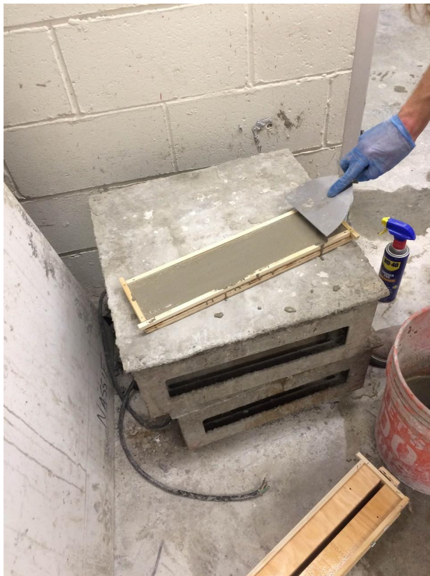
Figure 14: Trowel used to provide a smooth finish of the plate sample
