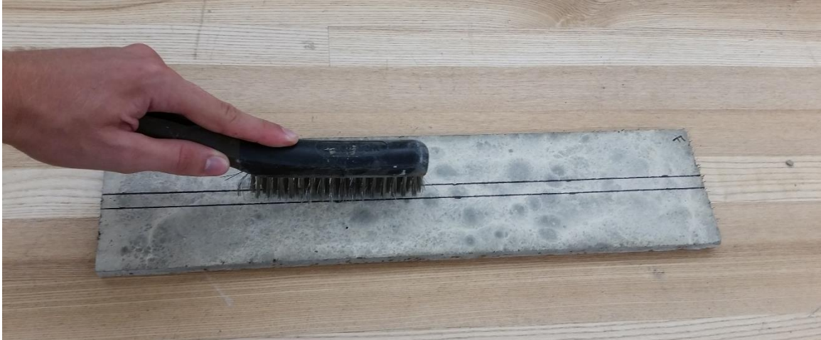
Figure 22: Steel brush producing a rough surface on the concrete plate
