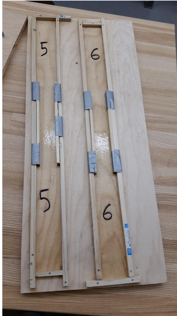
Figure 50: Molds for tension samples in third method
