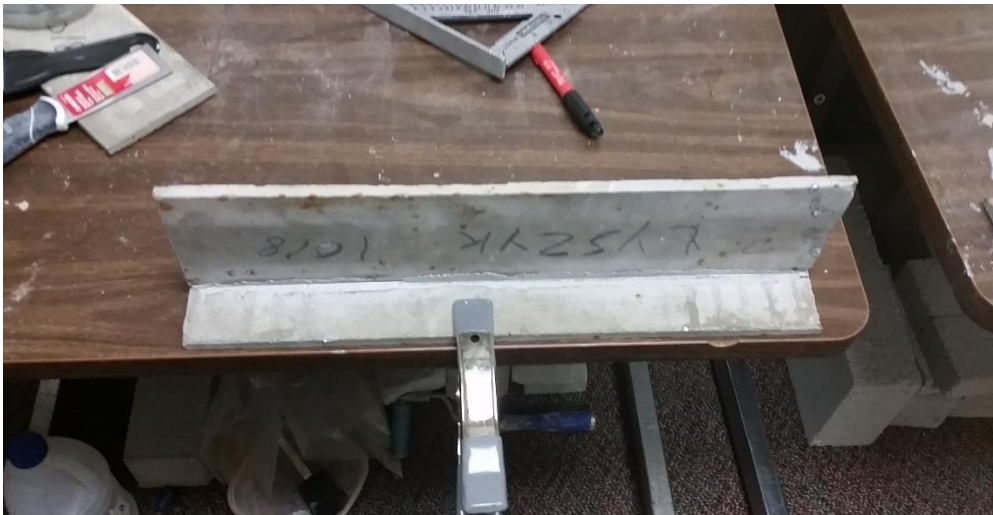
Figure 27: First flange to web attachment
