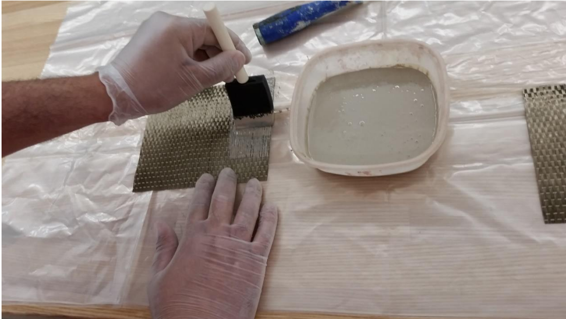
Figure 31: Brushing nano-inorganic composite onto basalt fiber
