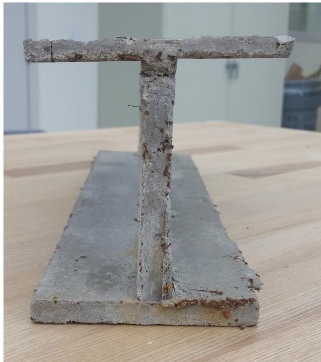
Figure 56: Misaligned web with bottom flange
