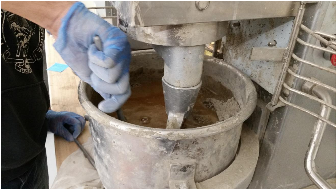
Figure 8: Creating voids prior for liquid to penetrate prior to wet mixing
