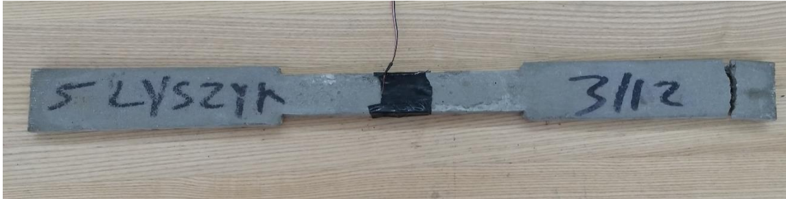
Figure 51: Failure occurred near grips for third method of tension test
