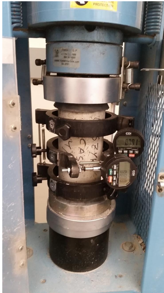
Figure 39: Cylinder in compression cage with elastic modulus cage
