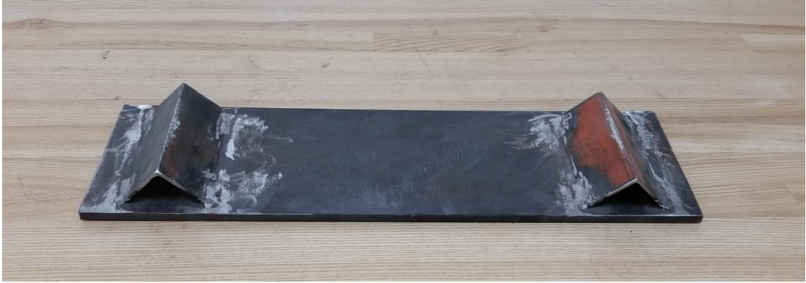
Figure 40: Simply supported system with two point supports
