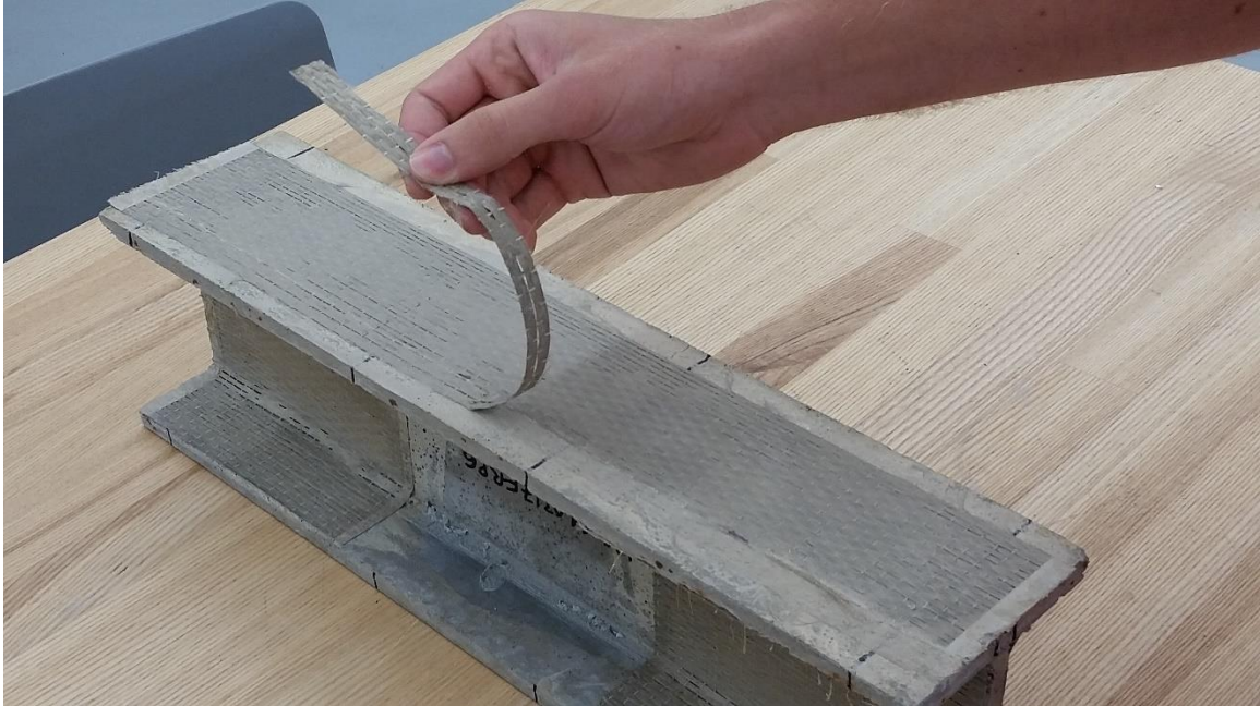
Figure 46: Removing a strip of basalt fiber
