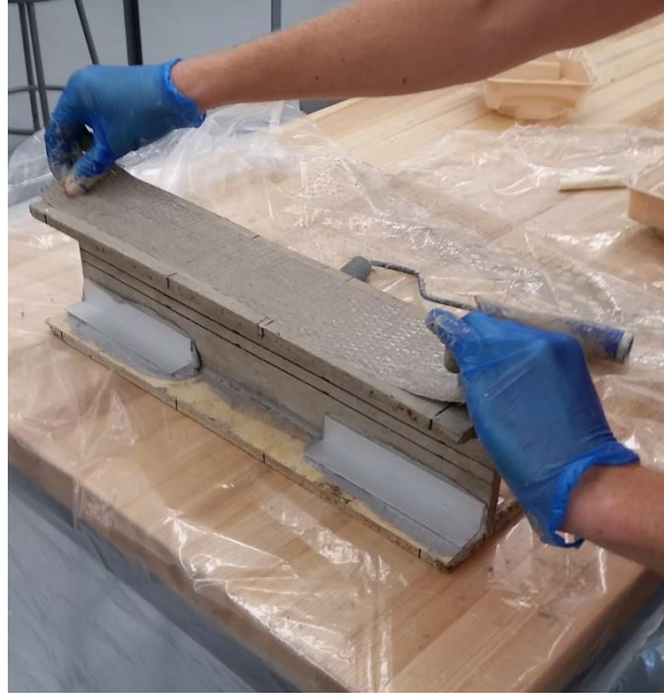
Figure 36: Aligning basalt fiber in the middle of the bottom flange
