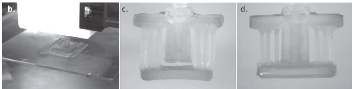
Figure 1-9 Printing process of the valve (left). The valve swollen in water at 20 °C (middle) and swollen in water at 60 °C (right) [39]
