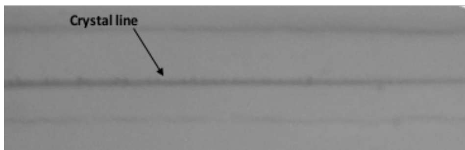
Figure 2-3. An optical image of the crystal line in the center of middle stream.
