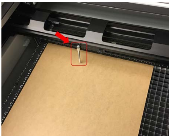
Figure D.10: Step 2: Focus the laser by adjusting the vertical height of the platform.
