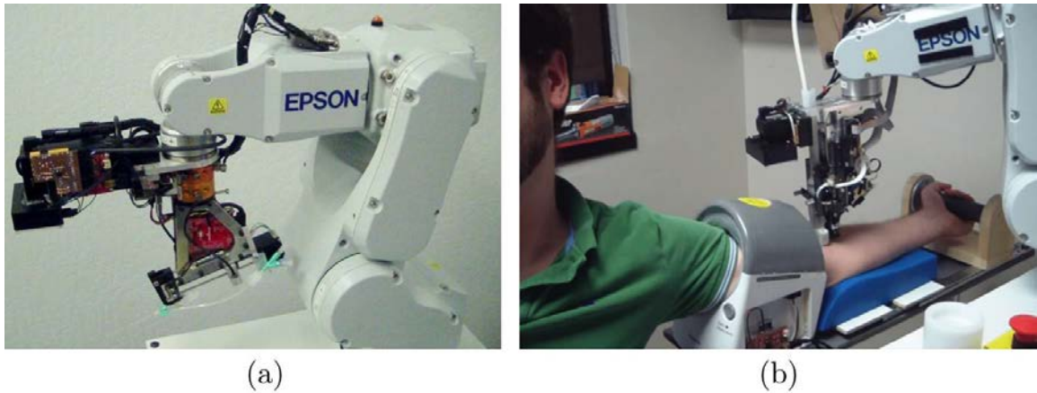
Figure 1.11: (a) The Veebot automated venipuncture robot, with the end-effector containing the imaging and needle insertion unit mounted on an industrial-sized robotic arm. (b) The Veebot performing a venipuncture on a human subject 142 .
