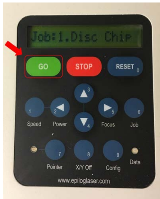
Figure D.23: Step 15: Press go on the control to panel to run the laser cutter.
