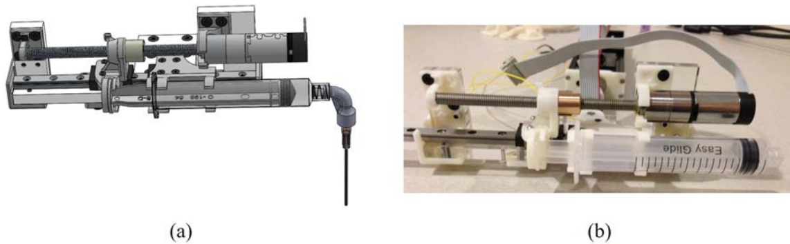
Figure 3.5: (a) Design and (b) prototype of the miniaturized syringe pump.
