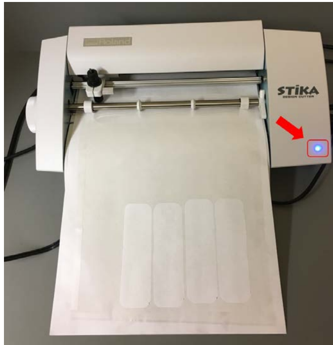
Figure D.24: Loading PSA (backed with a sheet of 8.5 x 11 in. paper) into the vinyl cutter. Blue LED indicates that the machine is powered on.
