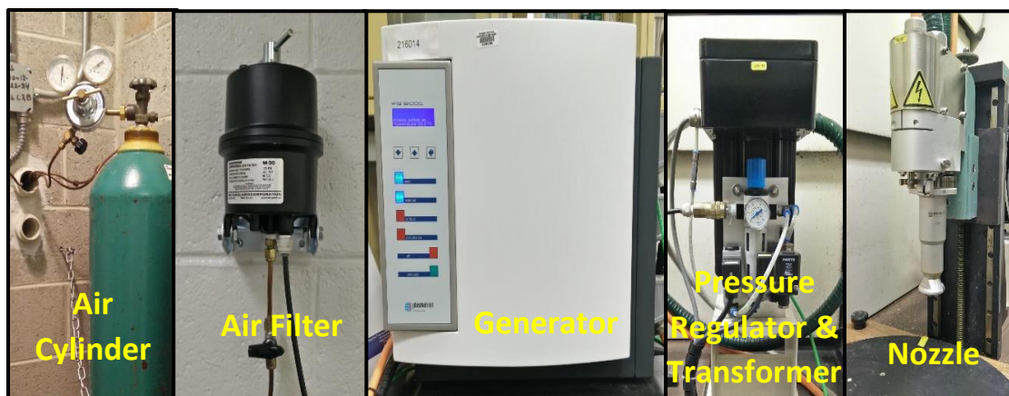
Figure 11: Setup of plasma unit at Rutgers University: Air cylinder, air filter, generator, pressure regulator, and nozzle.
