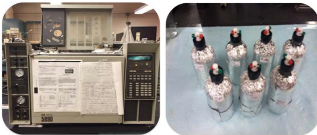
Figure 5. (Left) 5890A Hewlett Packed gas chromatograph; (right) 250 mL glass jars sealed with airtight valves for AITC headspace analysis.
