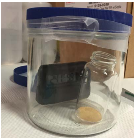
Figure 6. Monitoring the temperature and relative humidity (%RH) by using the mini-digital thermometer and hygrometer temperature humidity gauge.
