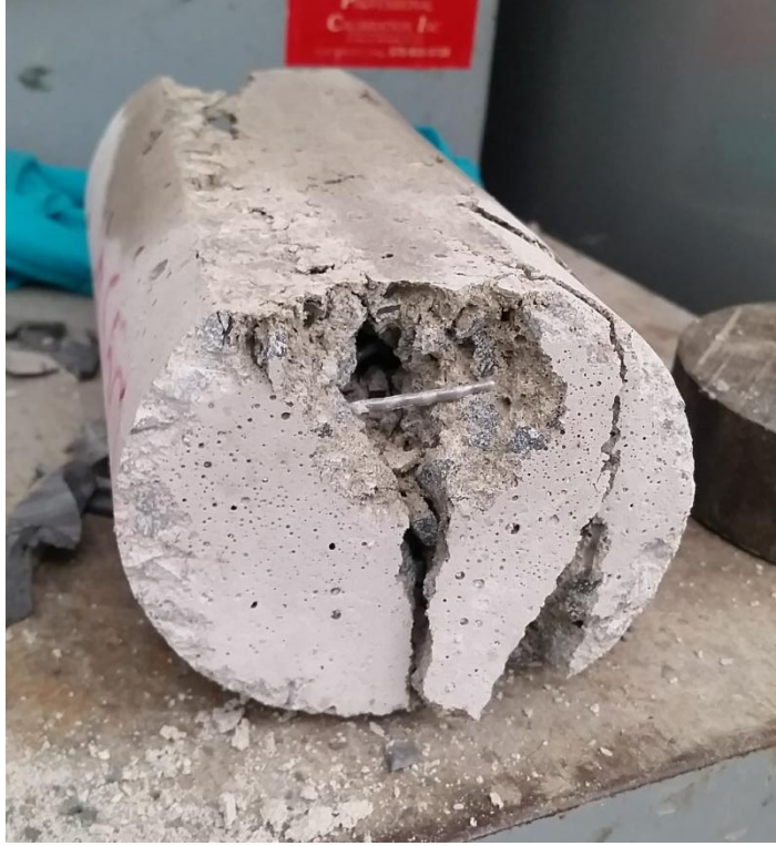
Figure 4.6 Deformation of FRSCC Under Tensile Splitting
