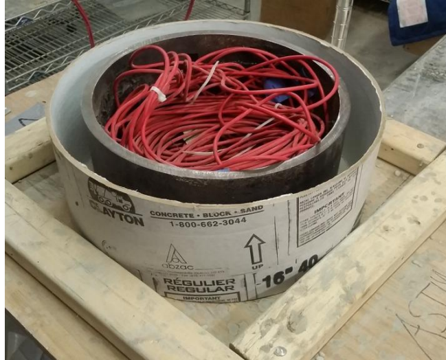
Figure 3.15 Final Setup for ASTM Ring
