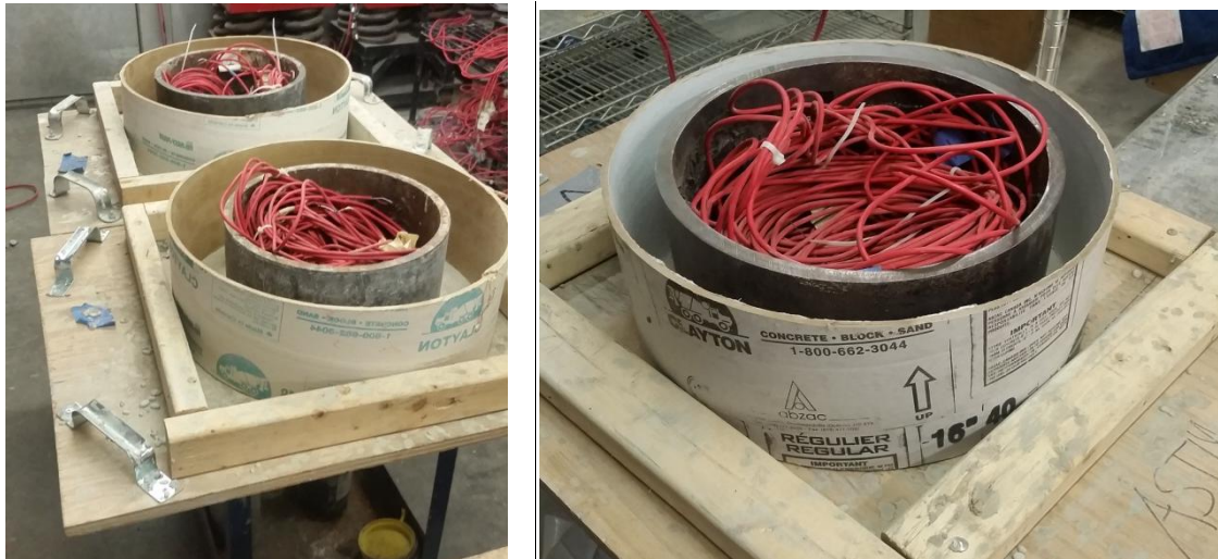
Figure 3.6 (a) AASHTO Ring setup (b) ASTM ring setup
