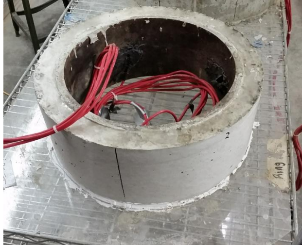
Figure 3.16 Final Casting and Placement of ASTM Ring
