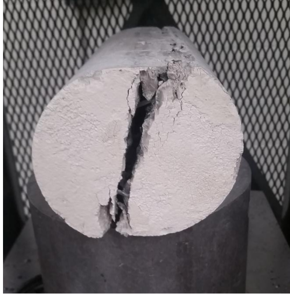
Figure 3.11 Splitting of FRSCC Specimen
