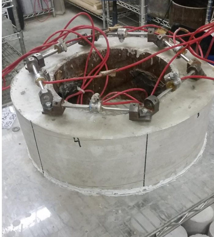
Figure 3.18 Final Casting and Placement of AASHTO Ring
