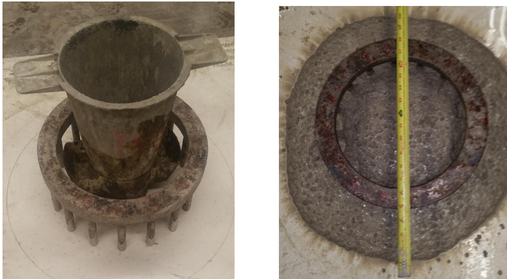
Figure 3.5 (a) J-Ring test (b) J-Ring flow
