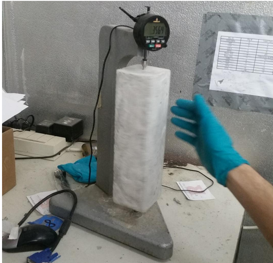
Figure 3.13 Free Shrinkage Testing
