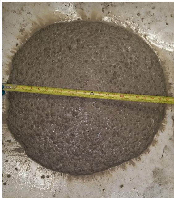
Figure 3.4 Measuring Slump (ASTM C1611)
