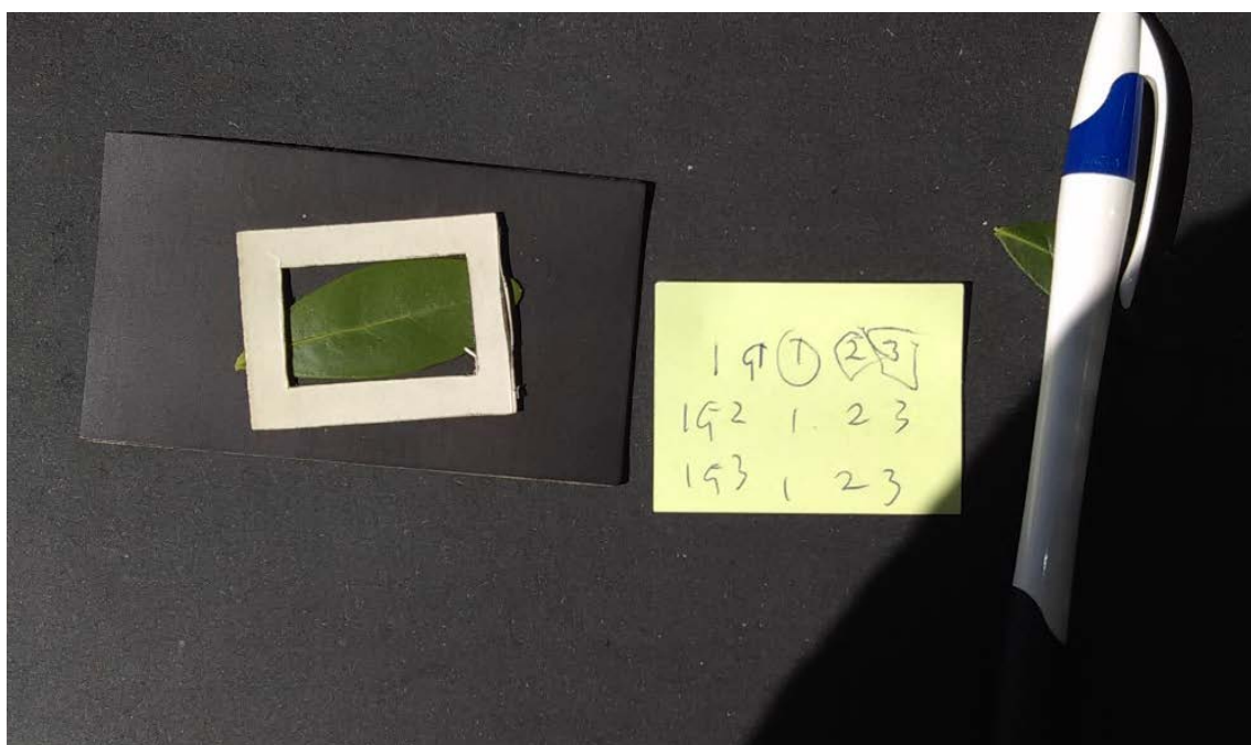
Figure 14: Photograph of leaf used to find ratio of leaf to cuvette area in LI-6400. Photo by author
