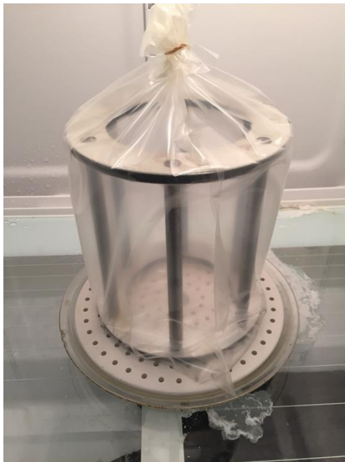
Figure 4.9 Setup of experiment for testing PVA permeability to ethylene
