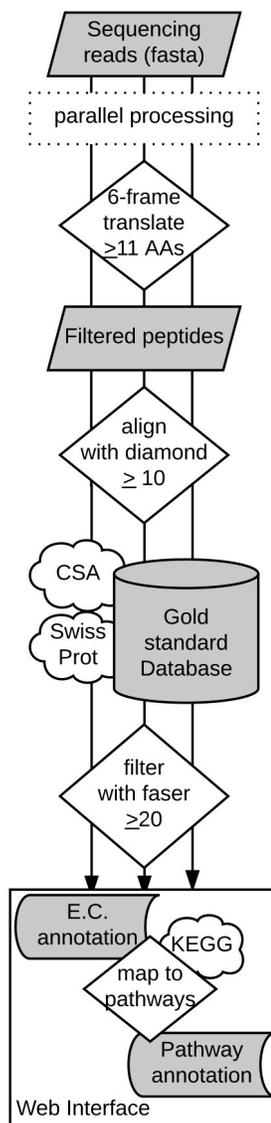
**Figure 4-1 mi-faser pipeline.** mi-faser is parallelized and runs a load balancer to submit jobs to available [1-2000] compute cores. Under normal functioning conditions (~400 available cores, onaverage), it takes ~30 minutes to process a single (10G/70M read) meta-genome/-transcriptome.
