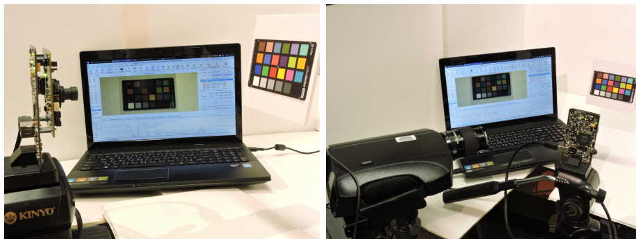
Figure 3.3: In the experiment, a CMOS digital sensor with 10-bit digital output was exposed repeatedly to a uniformly illuminated color checker. The figure shows the experimental setup.
