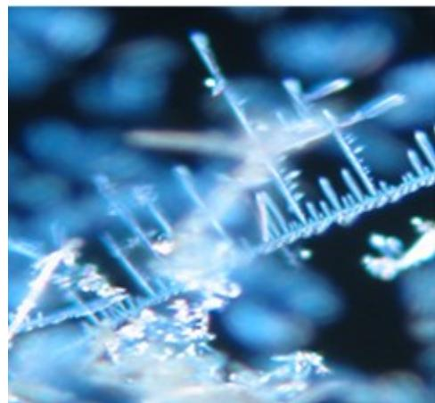
Figure 1-19. The precipitation product of the cocaine gold(III) chloride microcrystal test (mag. 40x).
