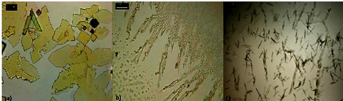
Figure 2-8. The precipitates of the HAuCl<sub>4</sub>- crystal test with a) amphetamine, b) ephedrine, and c) methamphetamine. Photomicrographs from the McCrone Research Institute.
