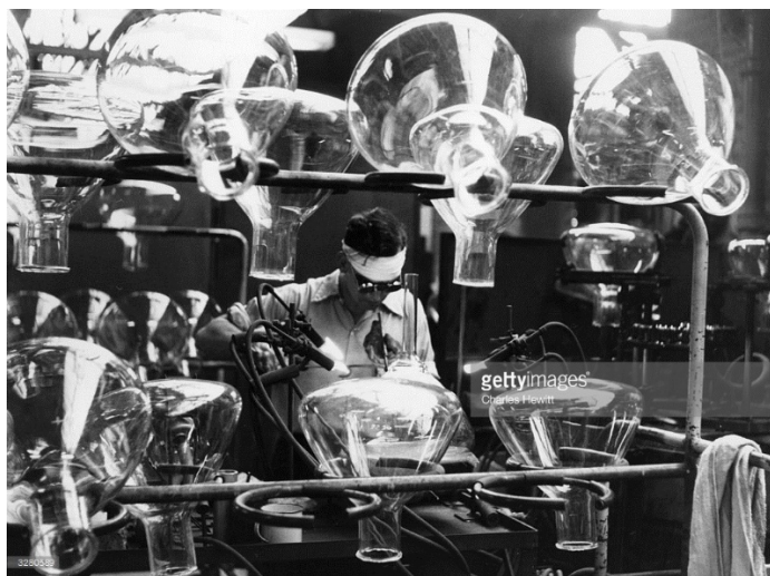
Figure 24. “Glassblowing television tubes in a factory,” 1955, gettyimages.com .
