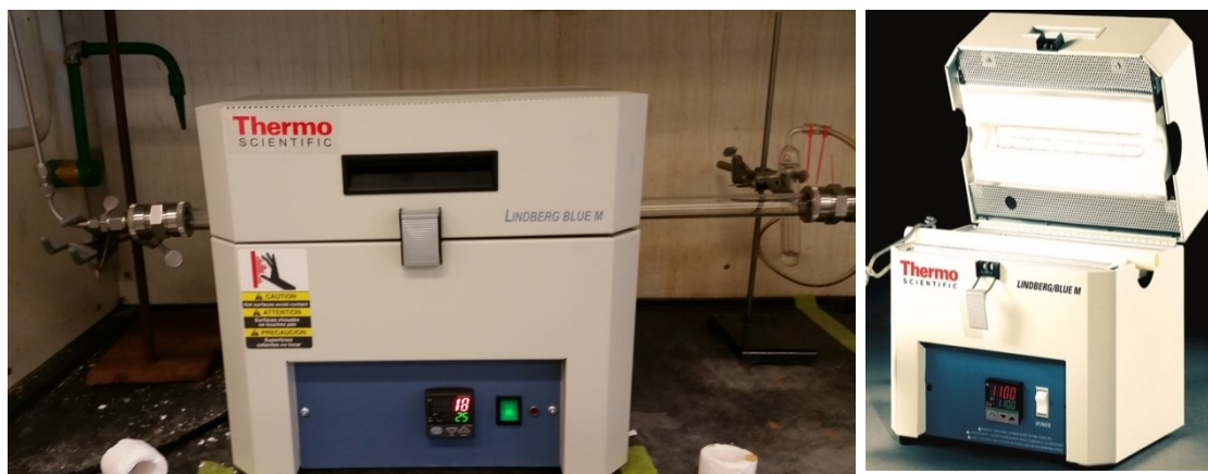
Figure 2.4: Experimental setup and image of Calcination furnace [Lindeberg Blue M] from Thermo scientific
